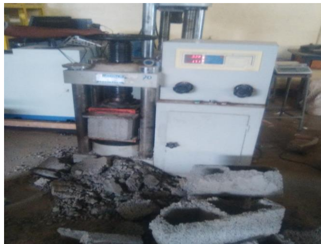
Figure: - 4.11 compressive strength test machine
