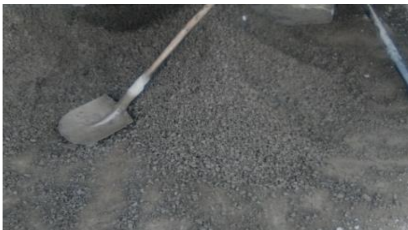
Figure 4.8:- HCB production by Hand mix
