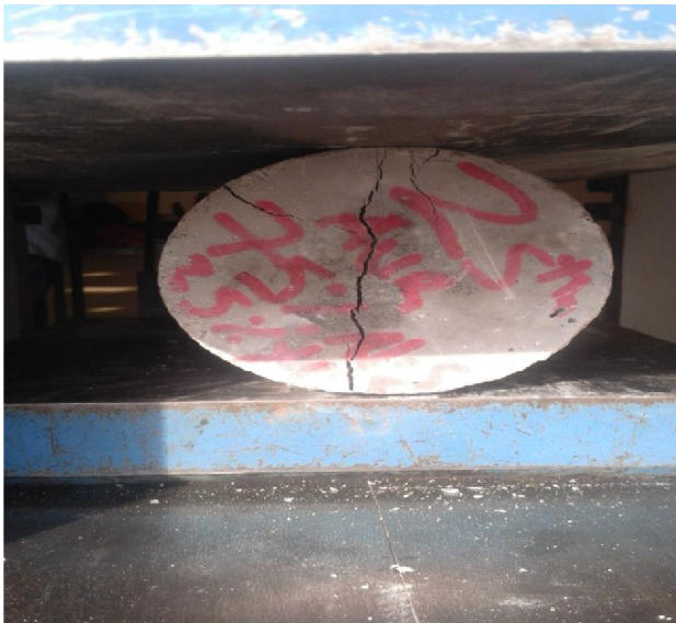
Figure 3.4 Split testing of cylindrical concrete
