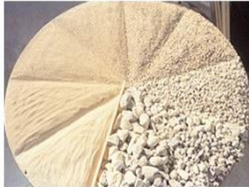
Figure 2.2 Range of particle sizes found in aggregate for use in concrete
