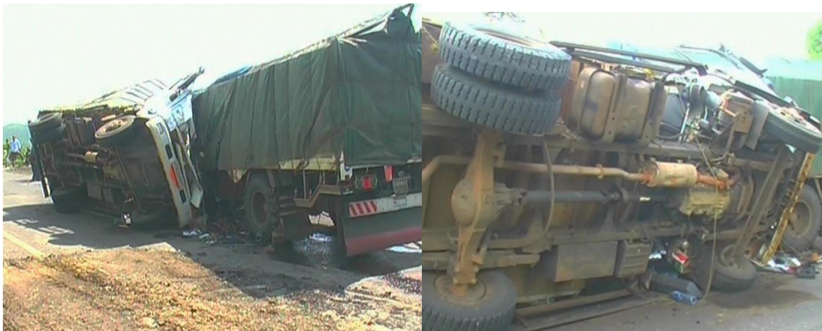
Figure 3.7: Accident occurred due to difficult down grade with worn-out pavement surface near to Dembeza Snt. Mary church.
