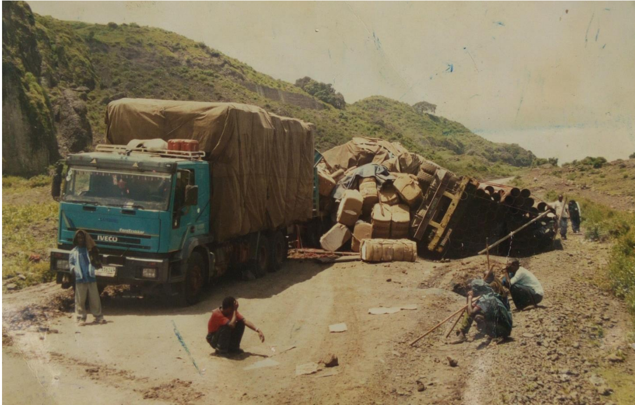
Figure 3.6: Accident occurred due to overturning at steep gradient of a curved section near to Bora Afaf (Source: Dejen woreda Police Communication Office).
