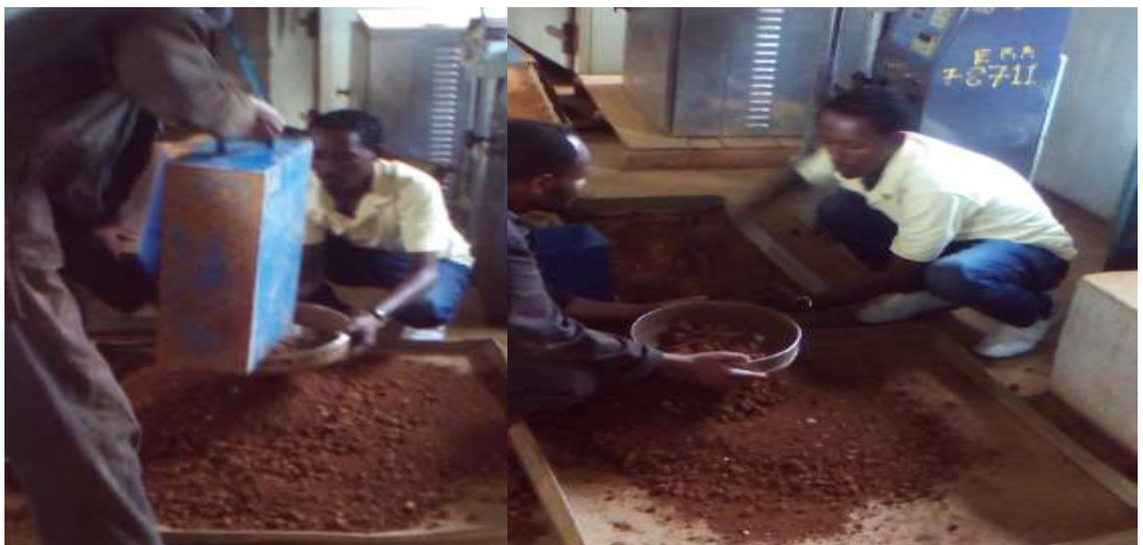
Sample preparation for laboratory tests by using sample splitter
