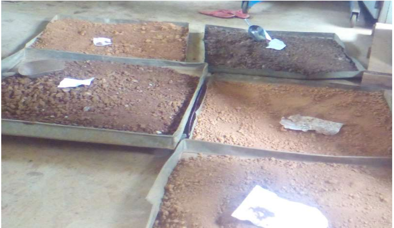
Sample preparation for laboratory tests by using sample splitter
