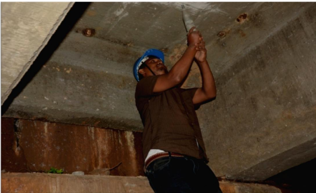
Figure 4.4: Smoothing with a carborundum stone of underneath deck test surface
