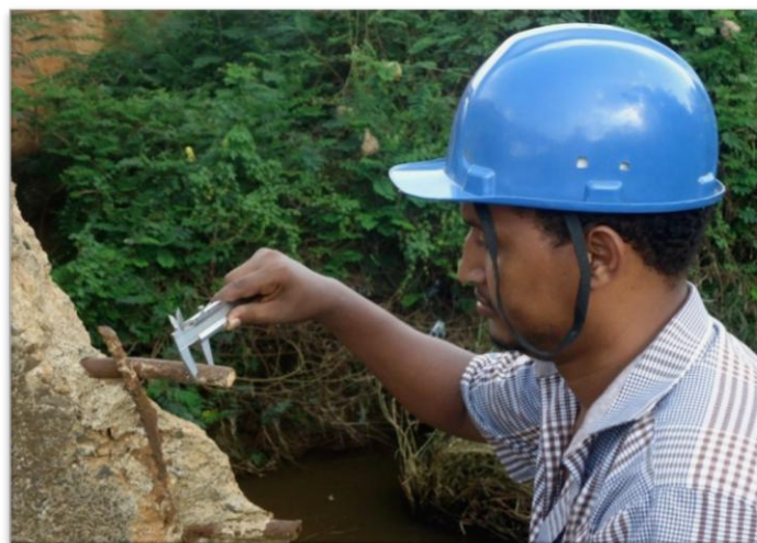
Figure 4.7: Measuring bare undeformed steel reinforcement bars
