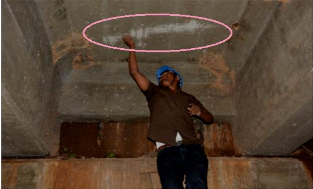
Figure 4.4: Smoothing with a carborundum stone of underneath deck test surface
