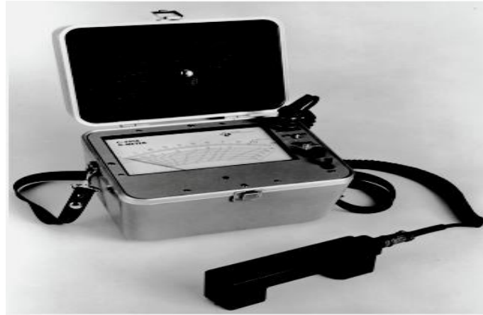
Fig. 2.7: Pachometer used to locate reinforcing in bridge deck [16]
