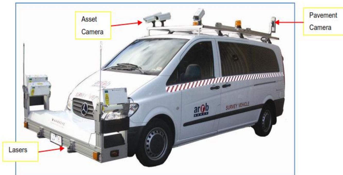
Fig.2.1: ARRB Automated Survey Vehicle (source: kassa;pavement performance evaluation)
