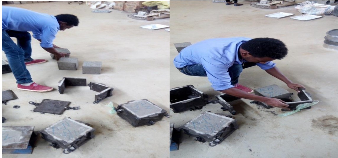
Figure 3. 7 Removing of concrete cube from the mold and immersion in to curing water.
