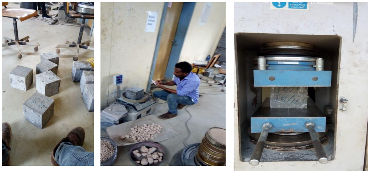
Figure 3. 8 surface draying, weighing and crushing of concrete cubes.
