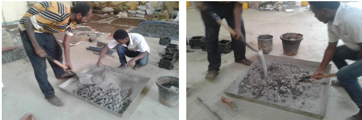
Figure 3. 5 Concrete mixing process.
