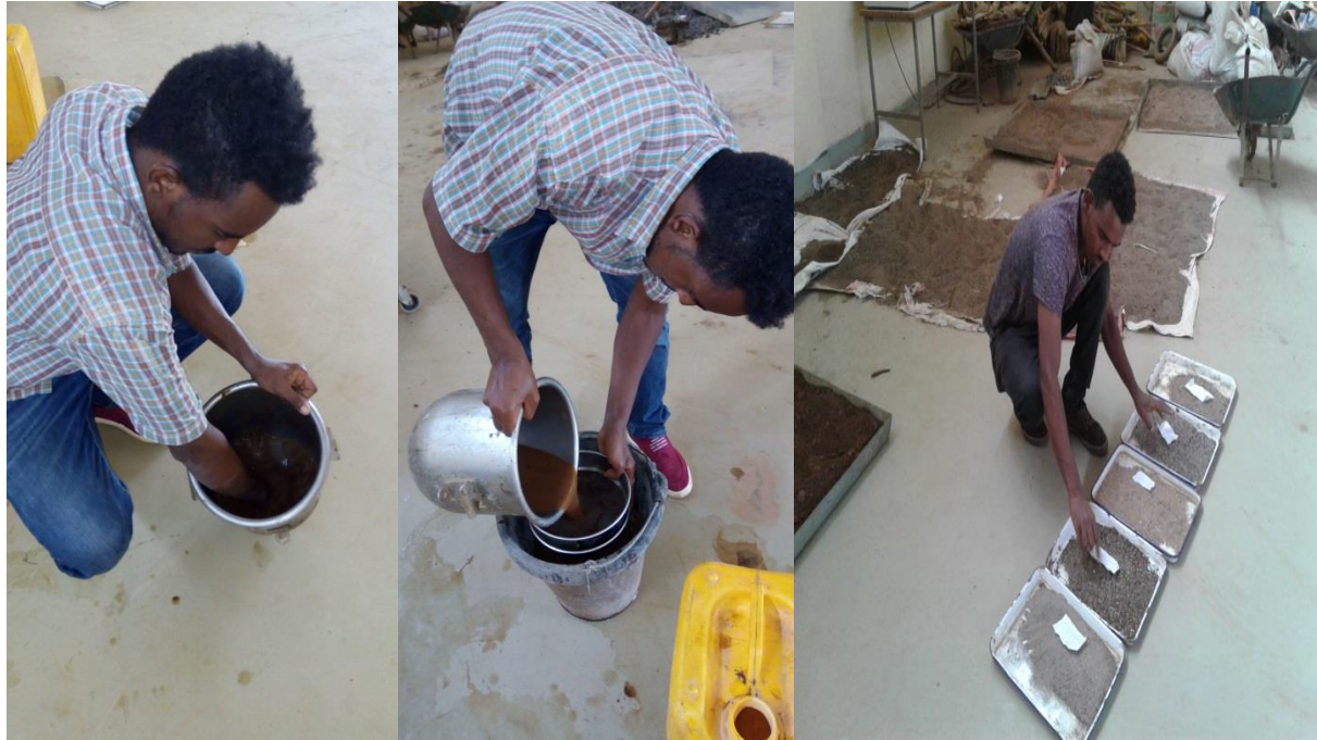
Figure 3. 4 Shows washing, wet sieving of sand on 75µm and oven dried sample.
