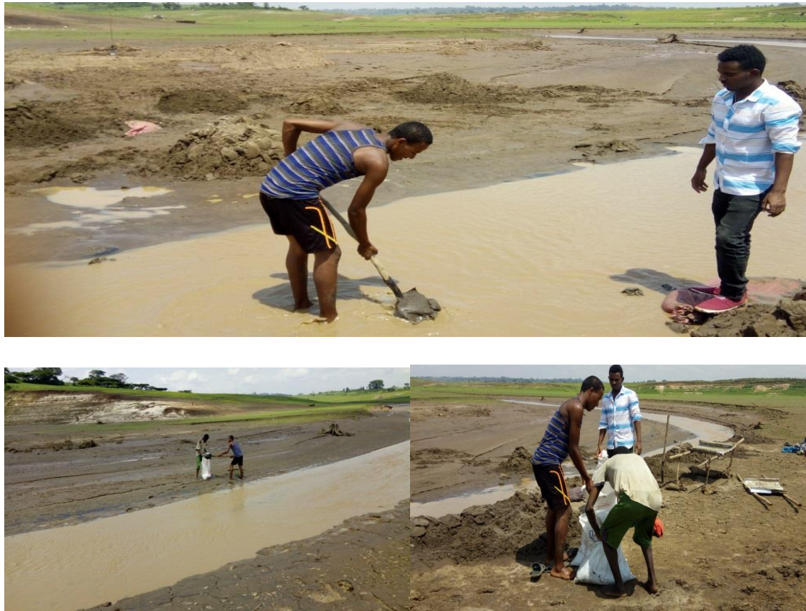
Figure 3. 1 Collecting representative sample from extraction site(river)
