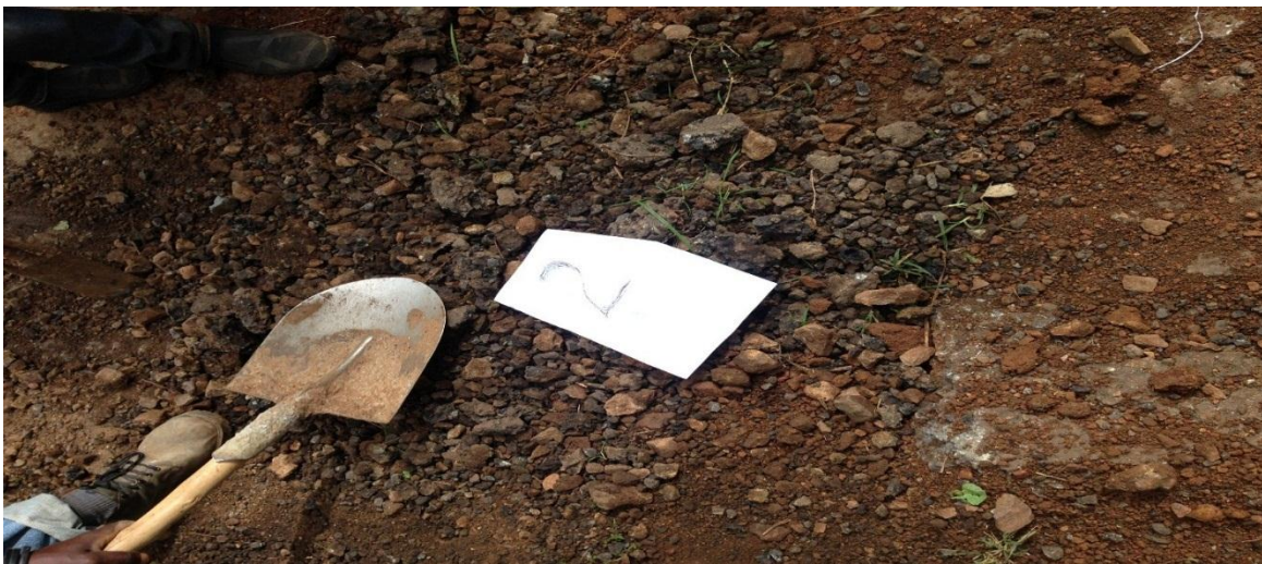
Reinstatement pit S2 after sample collected
