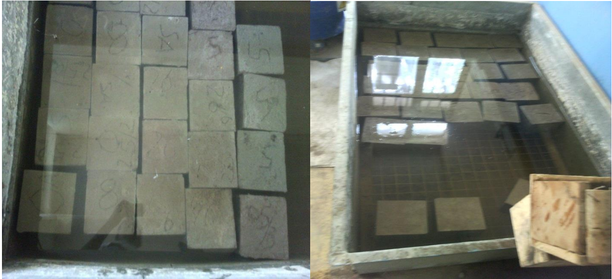
Cube cast of concrete during curing
