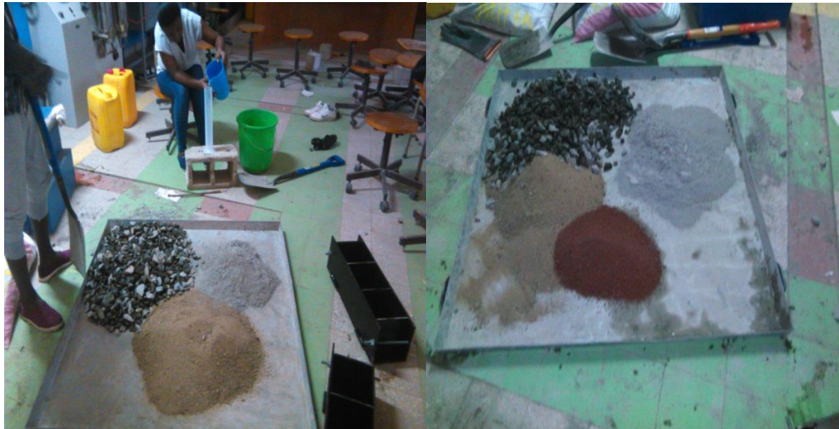
Prepared ingredients of concrete for mixing
