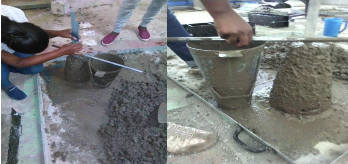
Slump test of trial mix
