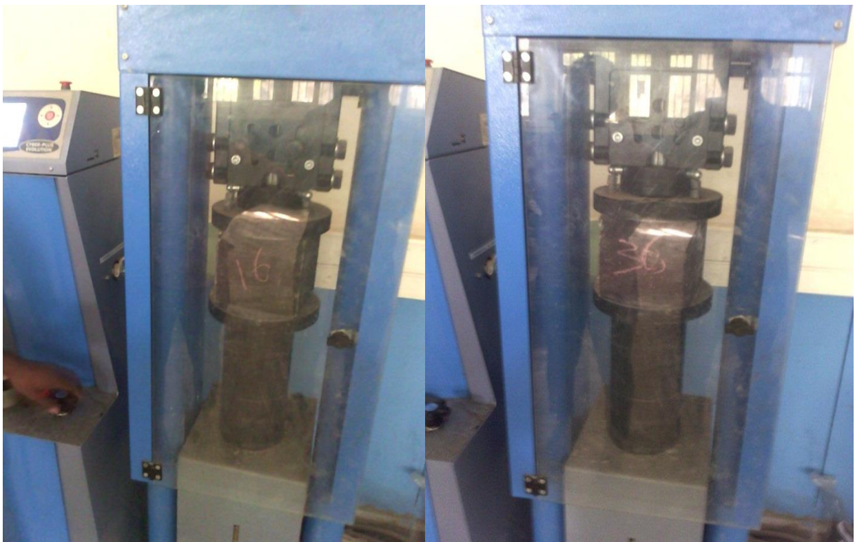
Fig 4 1: Sample prepared for test in compressive strength test machine
