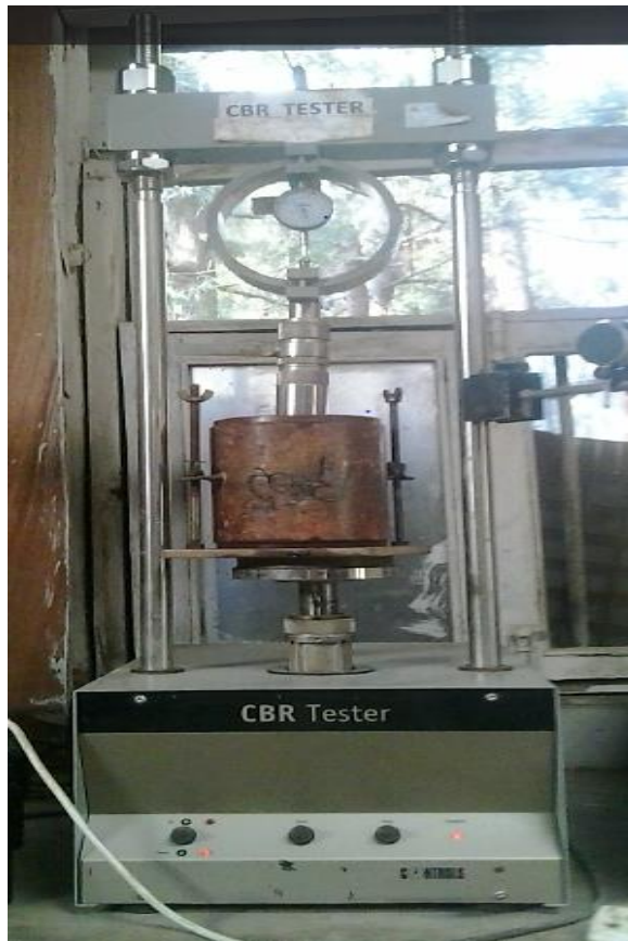
Figure 2.1: California Bearing Ratio laboratory Testing Apparatus
