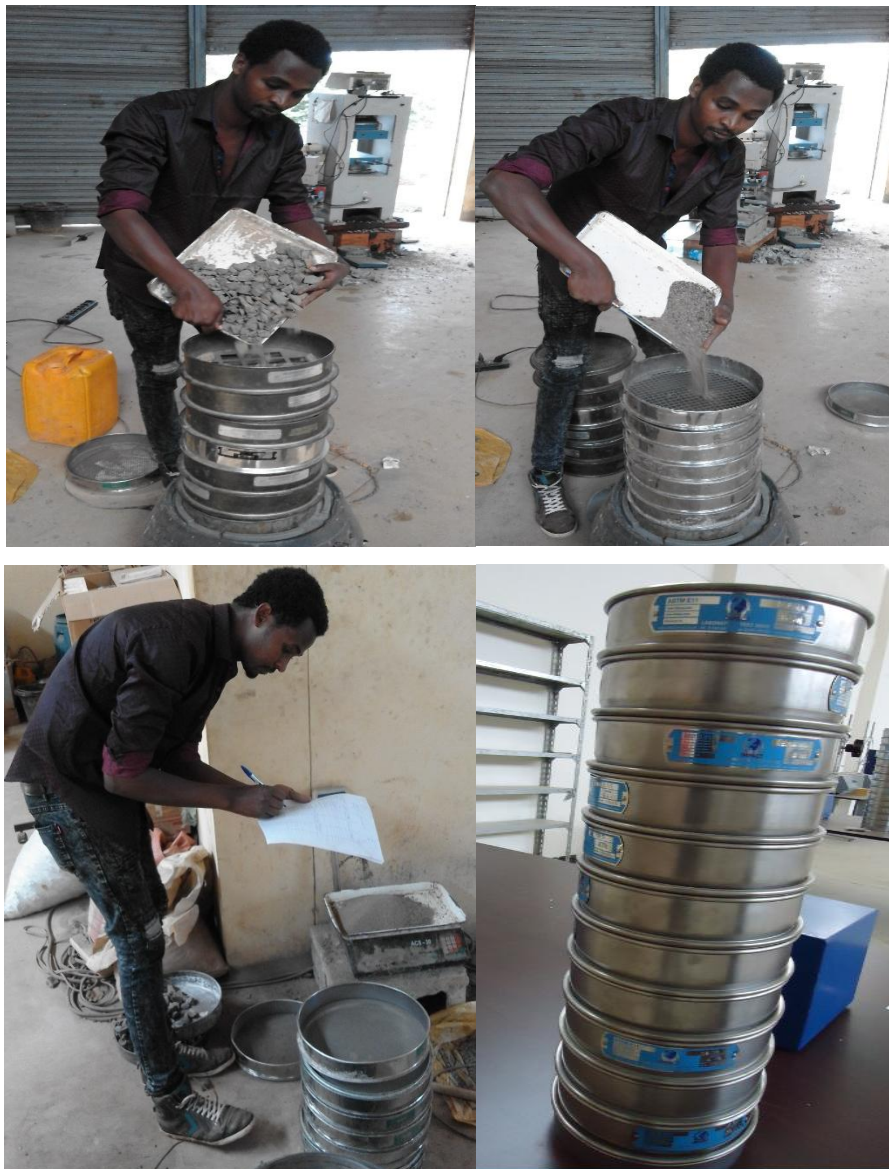
Figure 15:A Series of Sieves Standard Test Apparatus
