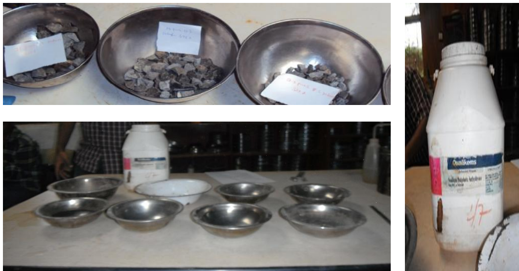
Figure 14: Soundness Tests by Sulphate
