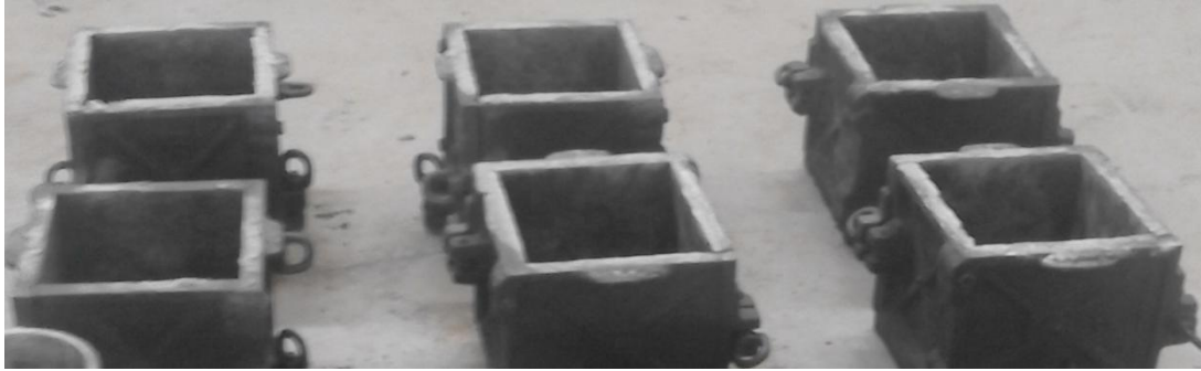
Figure 18: Typical 150 Mm Cube Mould
