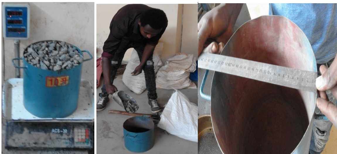
Figure 10: The Bulk Density of the Coarse Aggregate Test
