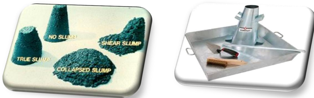
Figure 16: Scientific Standards for Slump Test Results.
