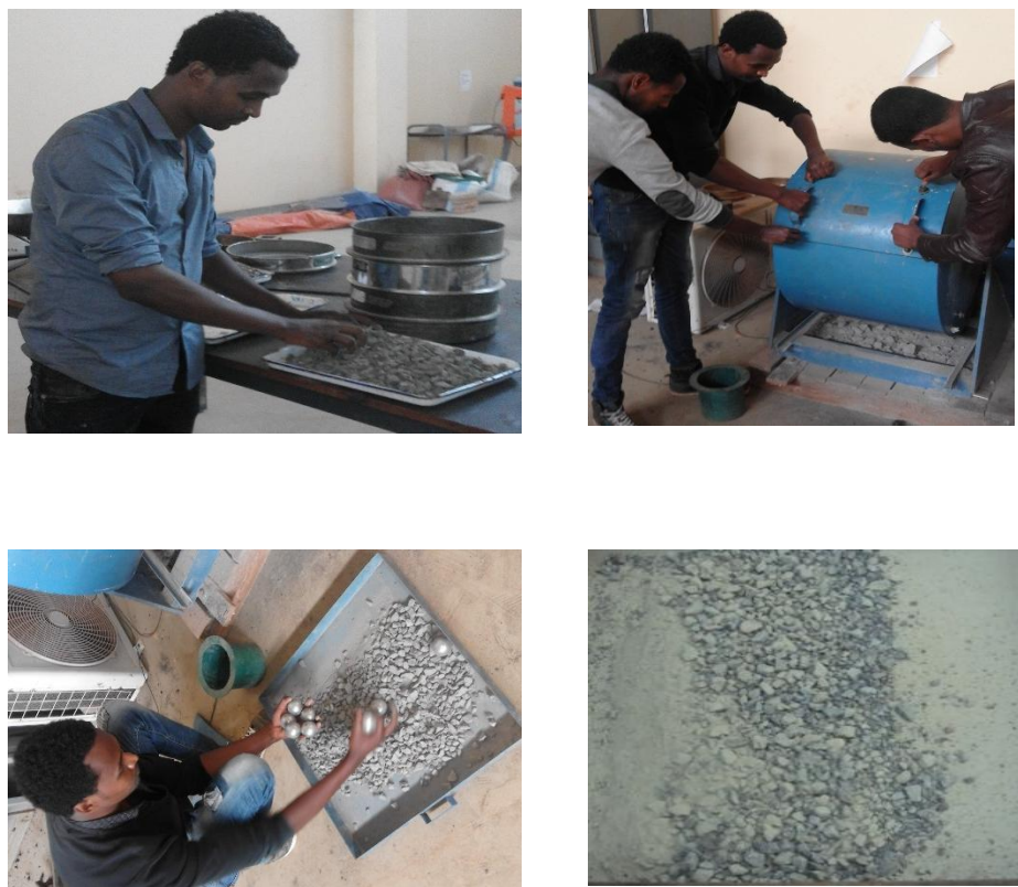
Figure 13: Abrasions and Impact in the Los Angeles Machine
