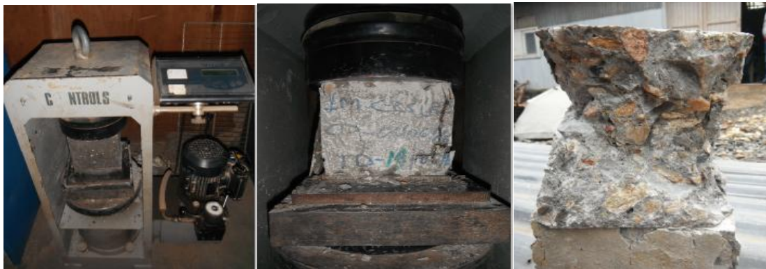
Figure 19: Compression Test Machine And Test Sample
