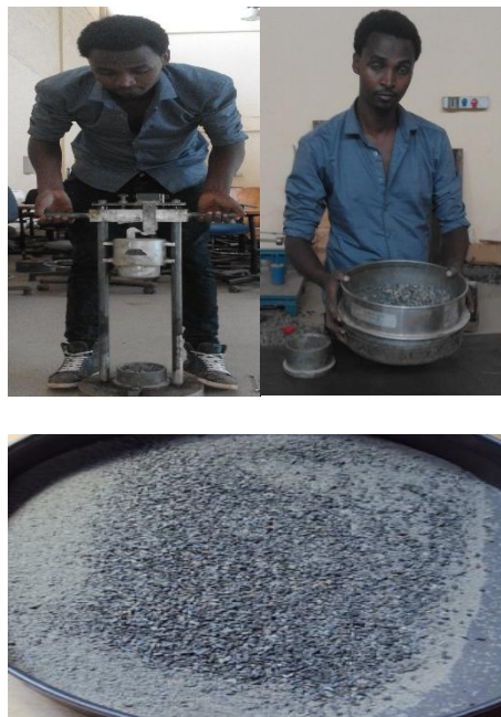
Figure 11: Aggregate Crushing Value (ACV) and test sample
