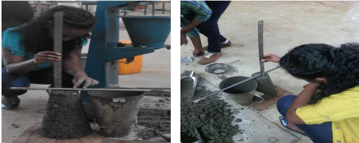
Figure 8.Measuring Slump of Fresh Concrete Mix
