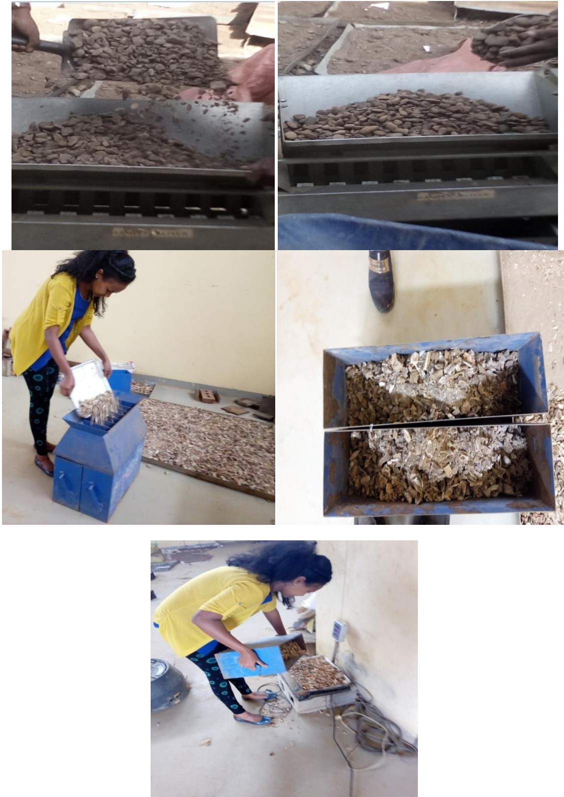
Figure 4: Reducing aggregate filed sample to test size
