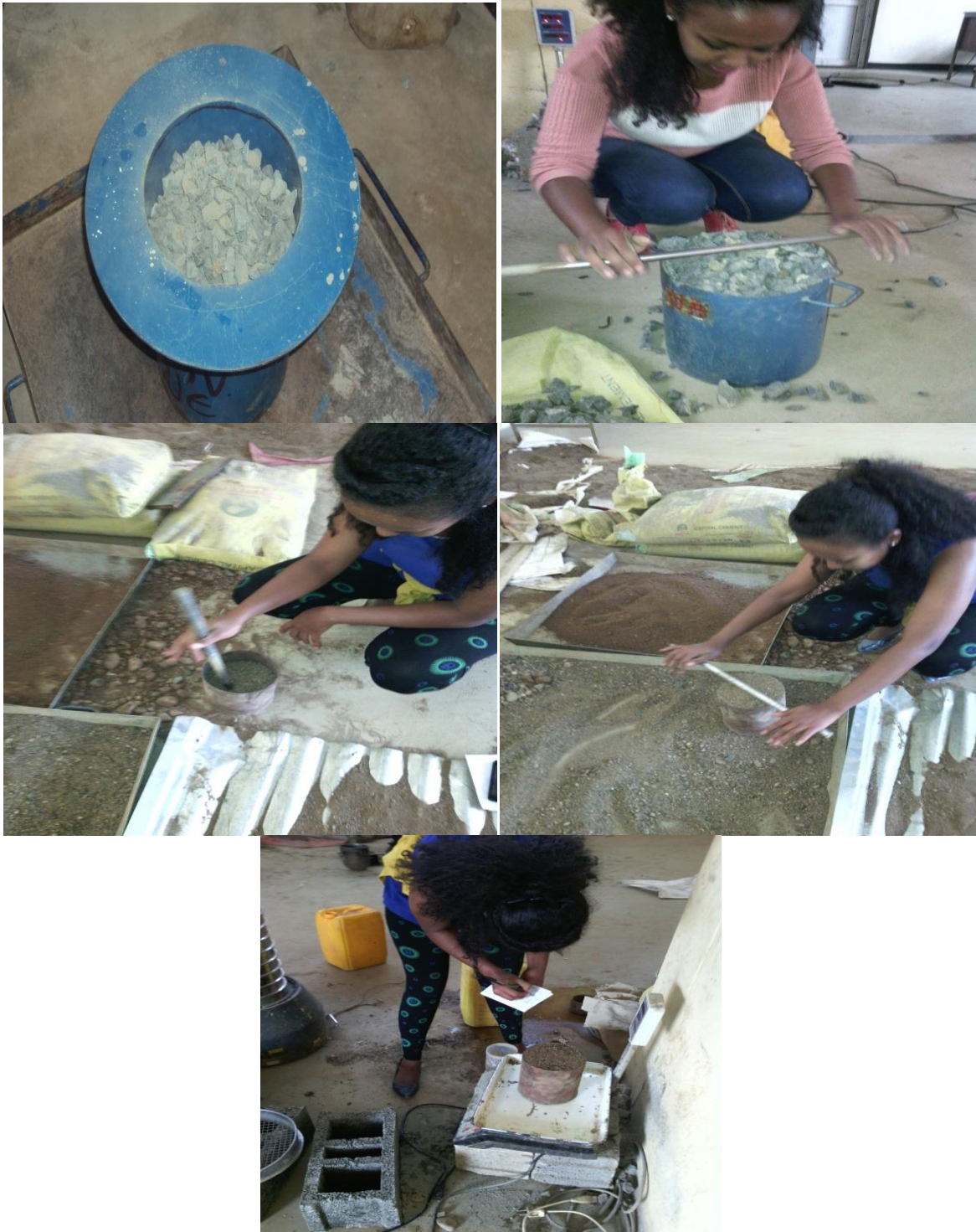
Fig7. dry rodded unit weight of aggregates
