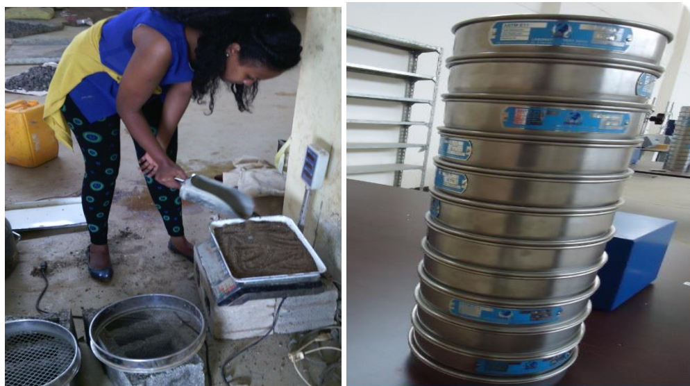
Figure 3.6 A Series of Sieves Standard Test Apparatus
