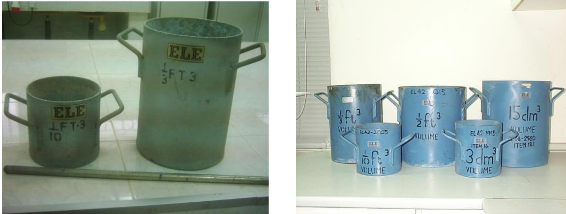
Figure 2.2 The Cylindrical Metal Measures for the Fine and Coarse Aggregates
