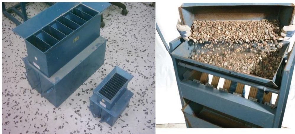
Figure 2.1: sample Riffing for fine & coarse aggregates to test size
