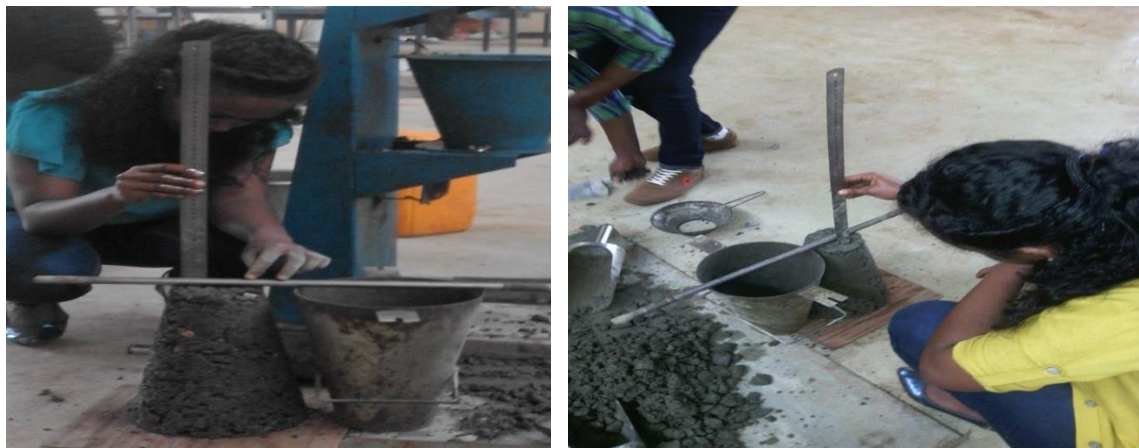
Figure 3.9 Measuring Slump of Fresh Concrete Mix
