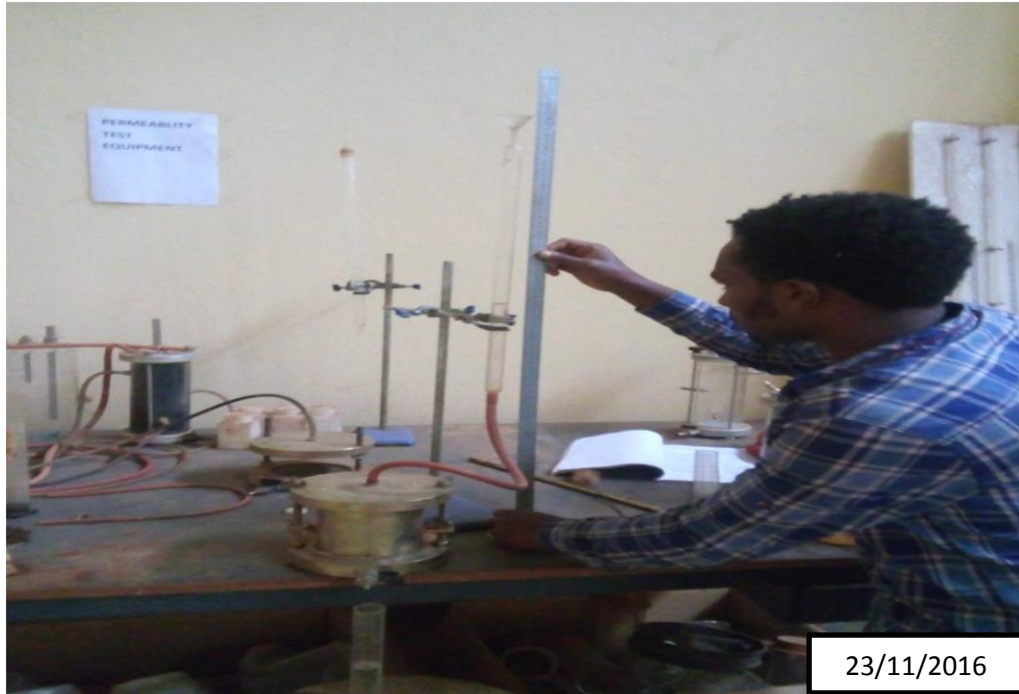
Figure 4.3: Falling head permeability (rate of capillary) test determination
