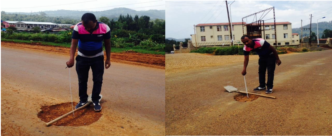
Figure 3.6 photos for measuring the Current Existing pavement Distress (Photos captured date15/04/2017@8:00 a.m. )
