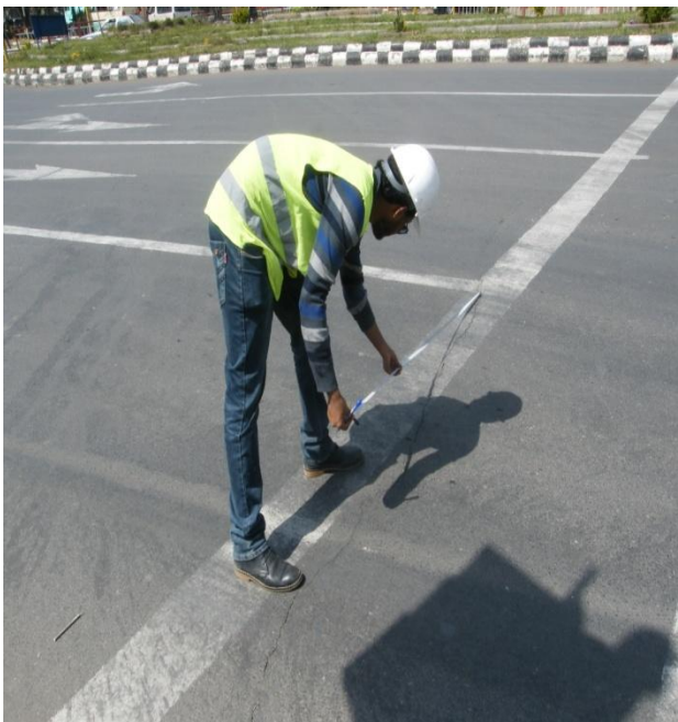
Fig.4.3 Photo: National Theatre 1 site: Measuring of crack size after the installation of the geogrid material
