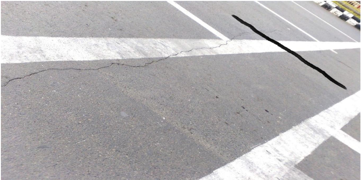
Fig.4.2 Photo: National Theatre 1 site: after 8 months of asphalt reinforcement. The Black heavy line represents the boundary between the control section and the reinforced section.
