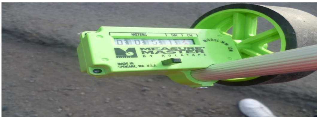
Figure 3.3 measuring wheel/Hand odometer wheel
