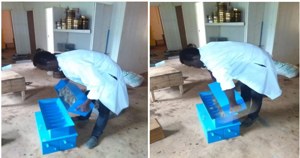
Figure 3-2: Sample splitting in laboratory for tests
