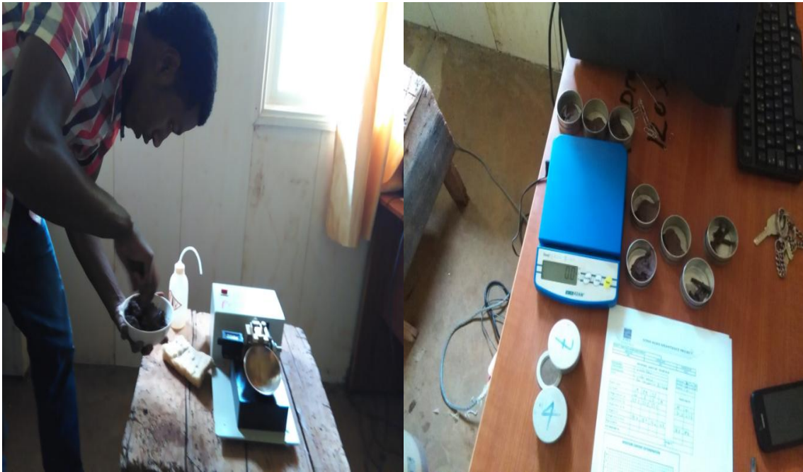
Figure 3-6: Laboratory test for Atterberg limit determination
