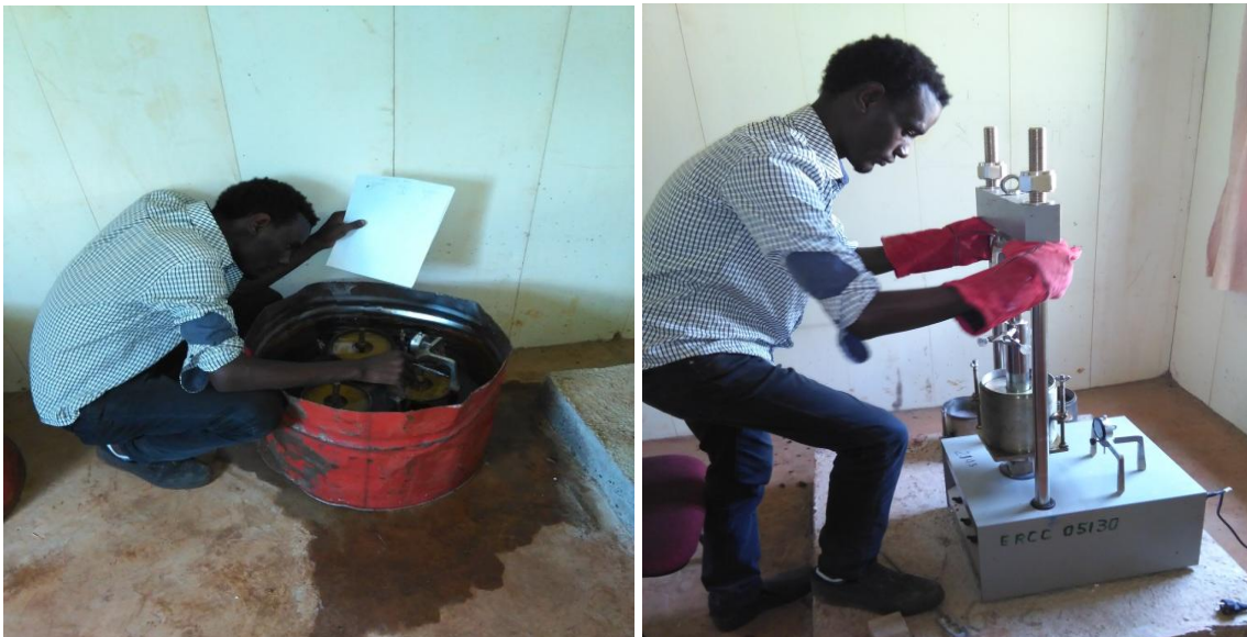
Figure 3-10: Laboratory test for CBR value determination
