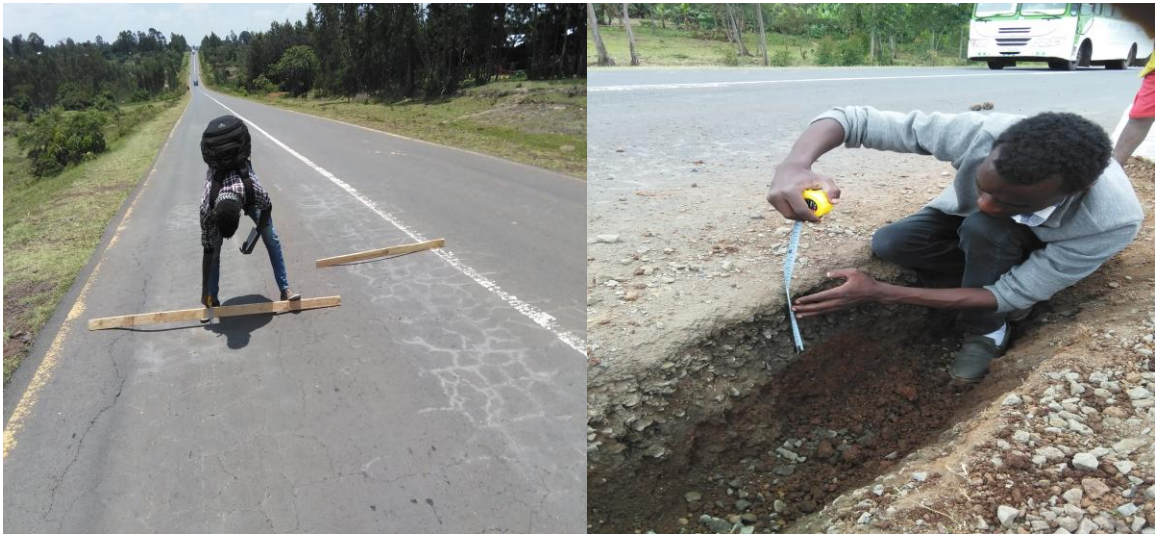
Figure 3-5: Shows the condition surveys and Measurement of thickness of pavement layers on sub section road Buge to Boditi.
