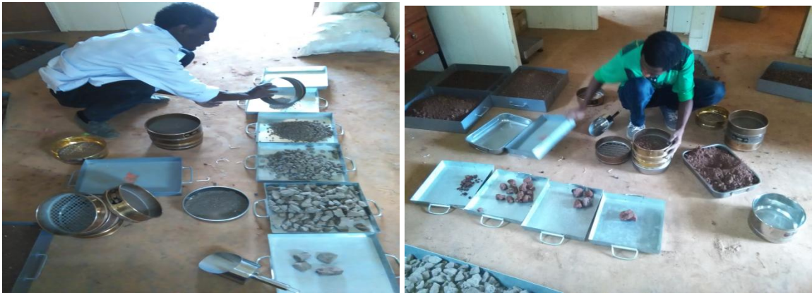
Figure 3-7: Laboratory test for grain size determination
