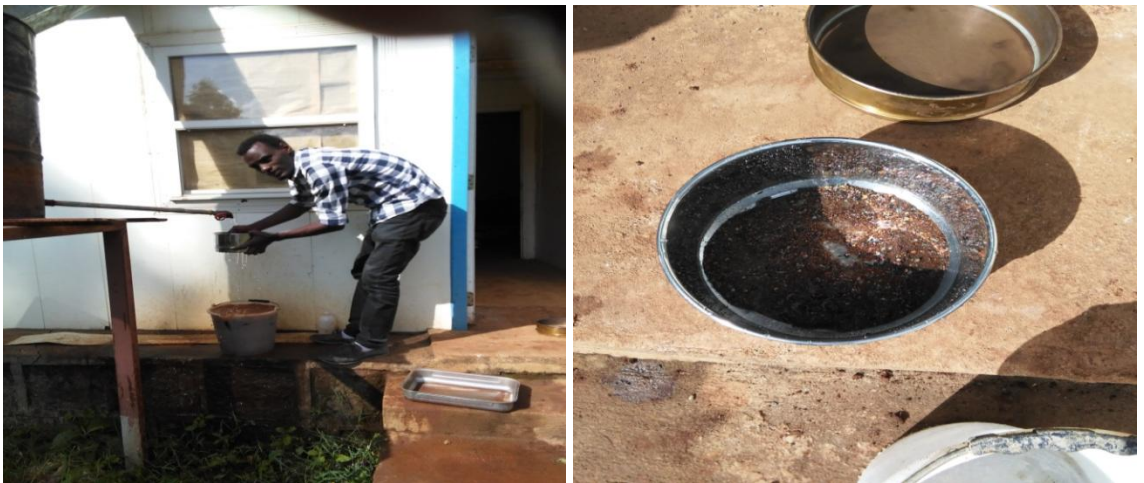
Figure 3-9: Laboratory test for soil classification determination
