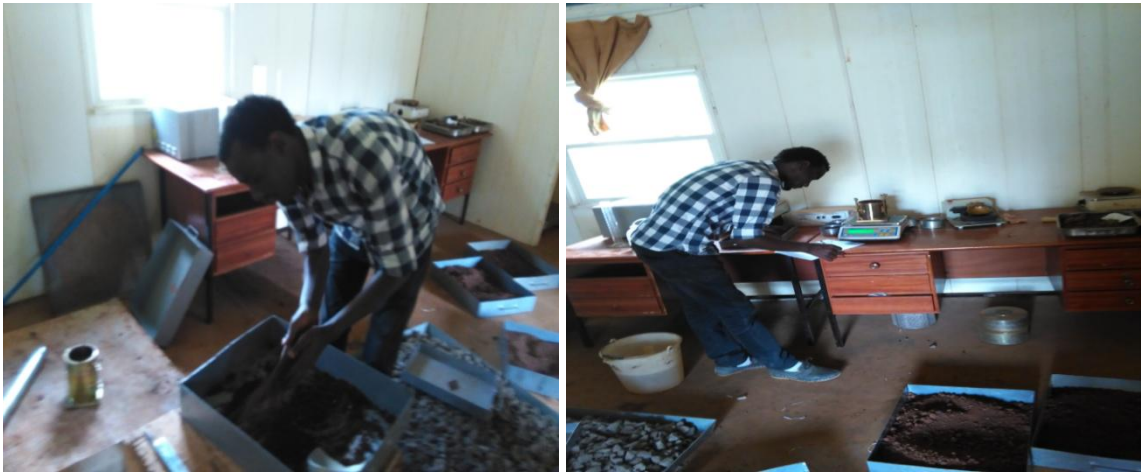
Figure 3-8: Laboratory test for MDD and OMC determination
