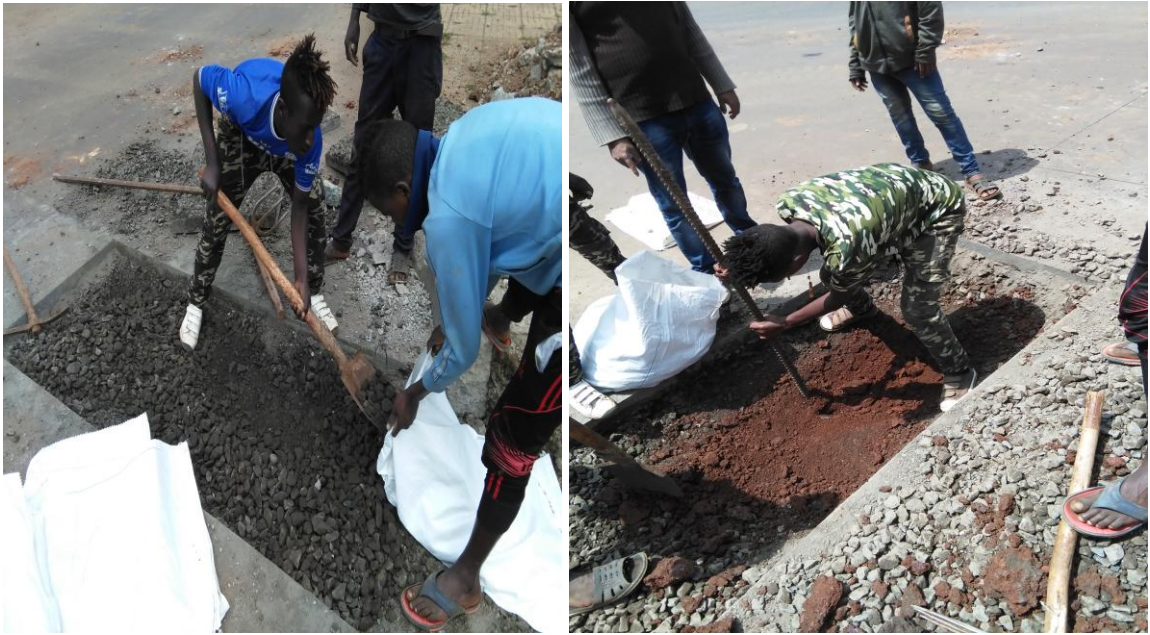
Figure 3-16: Sampling of subgrade soil, base course, and sub base materials from existing pavement at Station 67+926 (Sodo Town).
