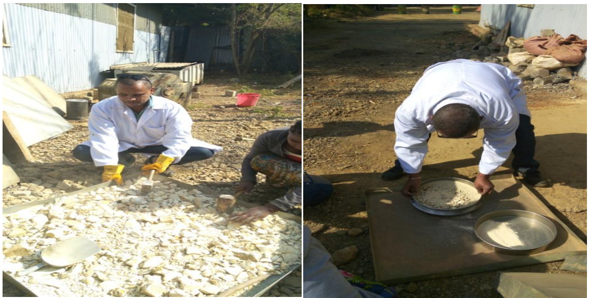
Fig. 4: Preparation for Lab Test of Physical Property of Natural subbase Material
