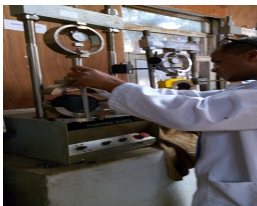
Fig. 7: Marshall Stability and Flow Test Machine
