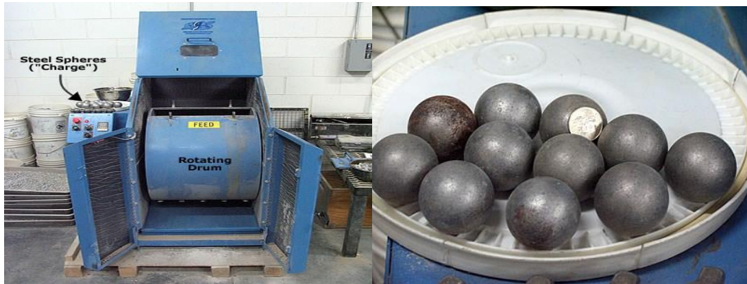
Fig. 3: Equipment Used for the L.A. Abrasion Test
