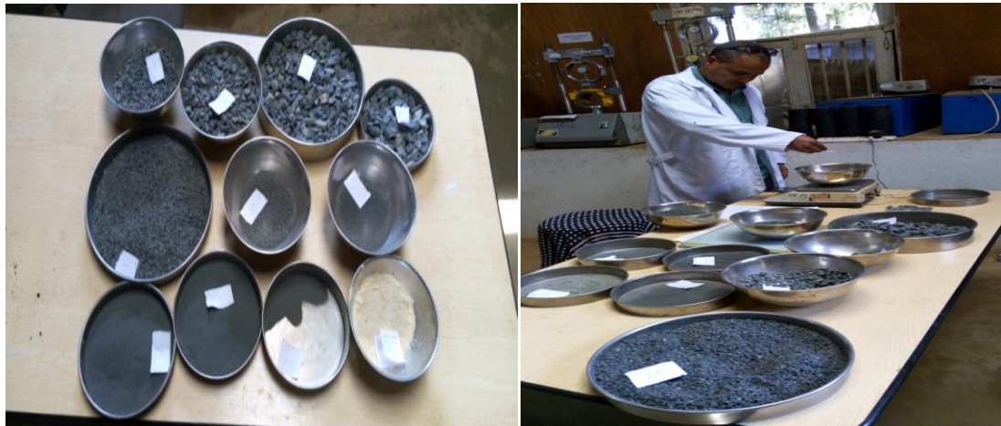
Fig. 6: Preparation of Aggregate for Specimen of Marshall Test
