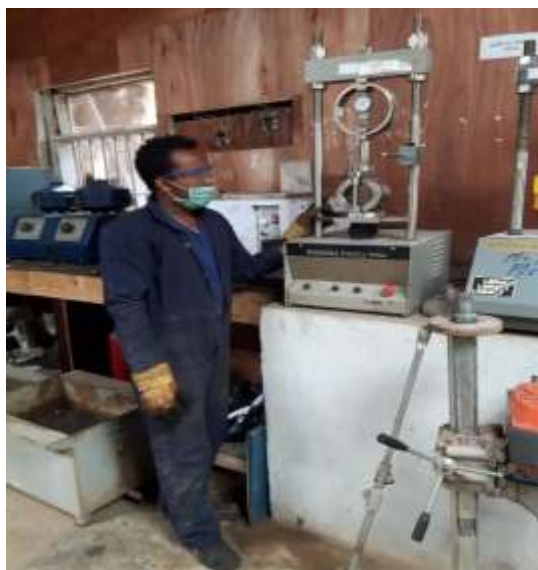
Figure 3.10: Marshall Stability and flow test machine
