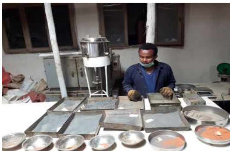
Figure 3.4: Preparation of aggregate for specimen of Marshall Test.
