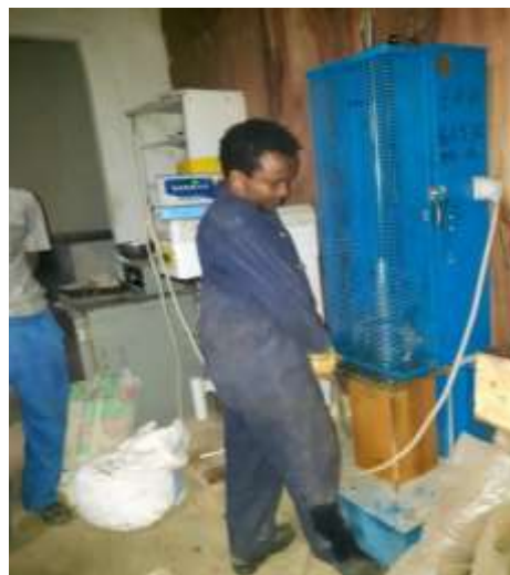
B) Compaction of specimens
