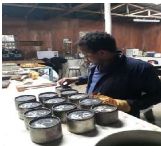
Figure 3.9: A) Packing the mold and Compaction of specimens allowed cooling
