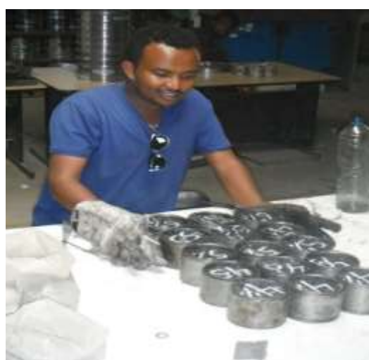
Figure 3.9: A) Packing the mold and Compaction of specimens allowed cooling
