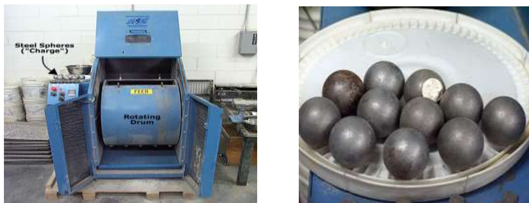
Figure 3.1: Major equipment used in the L.A. abrasion test.
