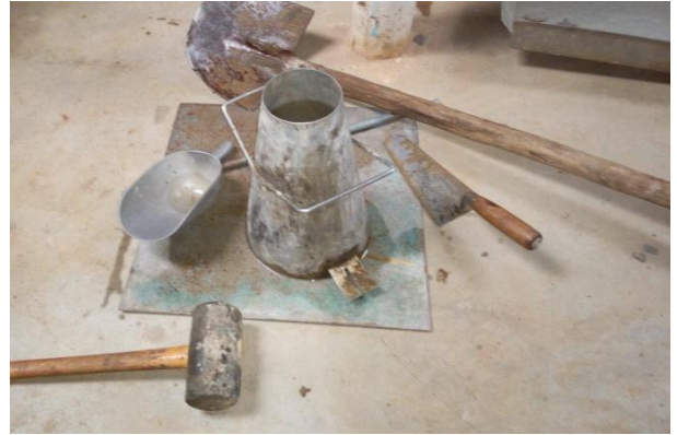
Equipment's used for slump test.
