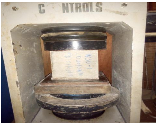
Cracking shape of C-25
