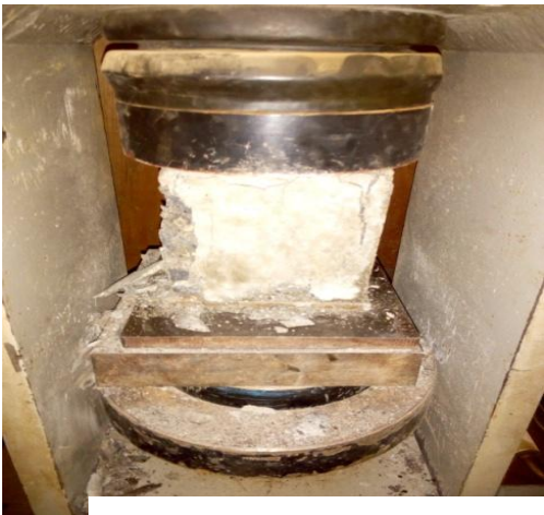
Cracking shape of C-40 PPC
