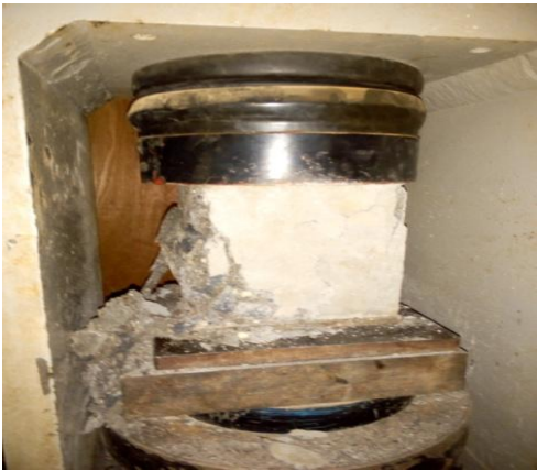
Cracking shape of C-25
