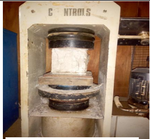
Cracking shape of C-40 OPC
