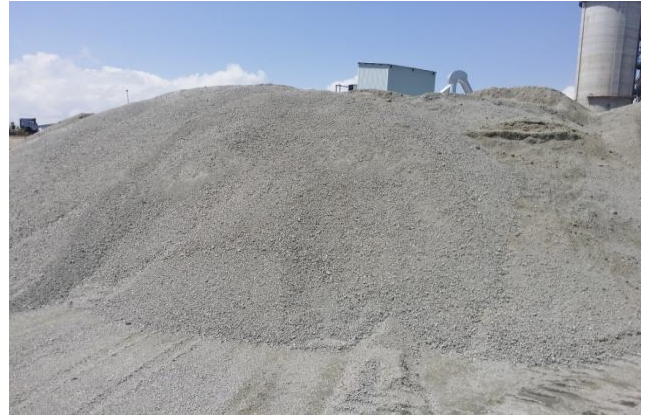
Crushed Gypsum ready for proportioning
