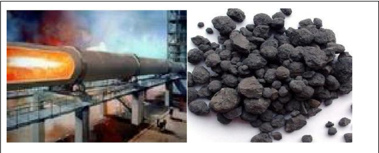
Figure 2.3: Burning the mixture in the kiln and formation of Clinker
