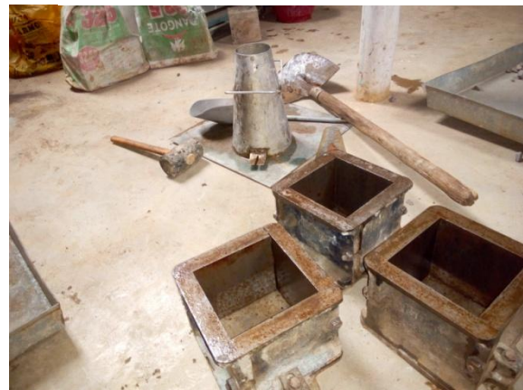
Cubical molds used for Concreting
