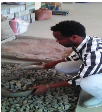
Sieving of aggregates during material preparation.
