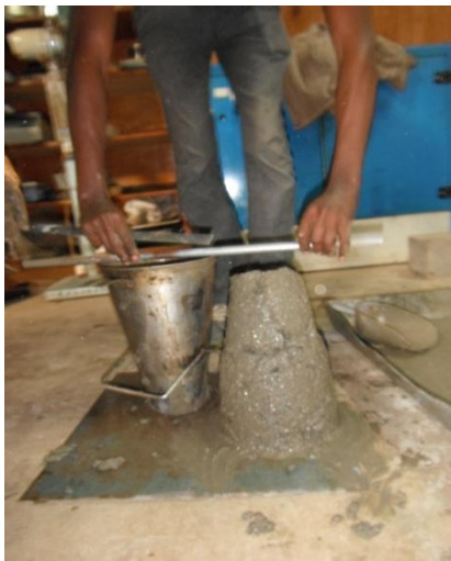
Slump test of Concrete
