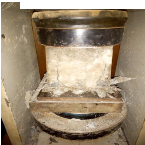
Cracking shape of C-70 OPC
