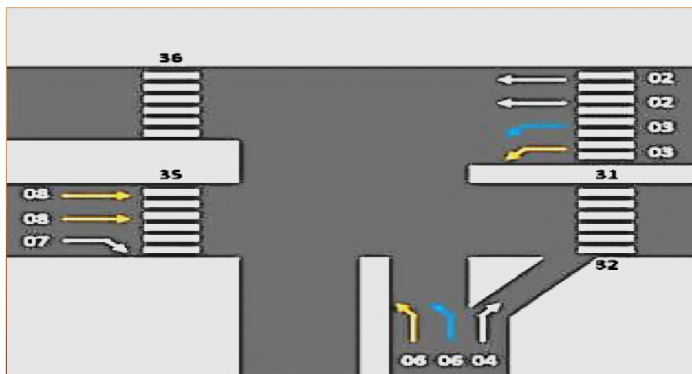
Figure 4.7: Lanes Layout of Un-signalized T-intersection, Wellosefer intersection
