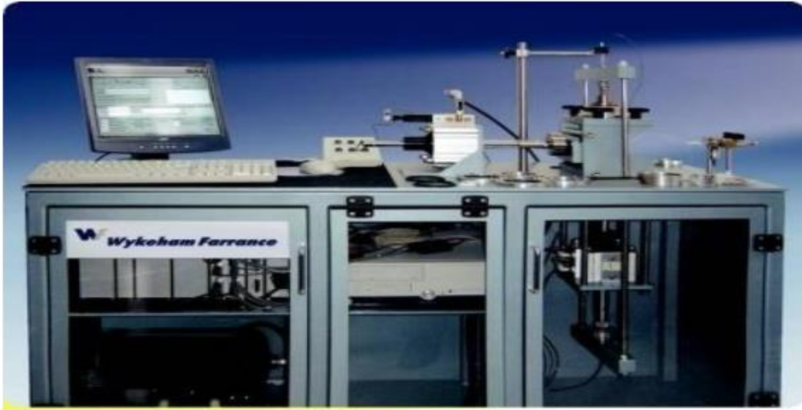
Figure 3-3: 31-WF7500 cyclic simple shear machine [26]
