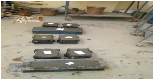
Photo: during casting of concrete and curing of concrete
