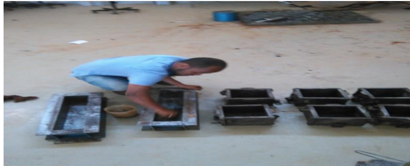
Figure 3- 4 lubricating of molds
