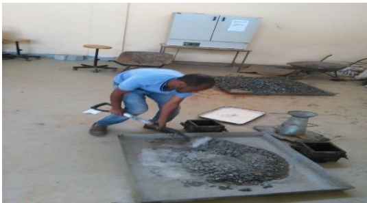
Photo: during mixing and slump test of concrete
