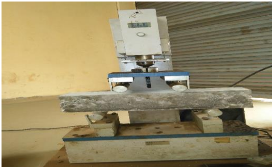
Photo: During before and after testing of flexural strength
