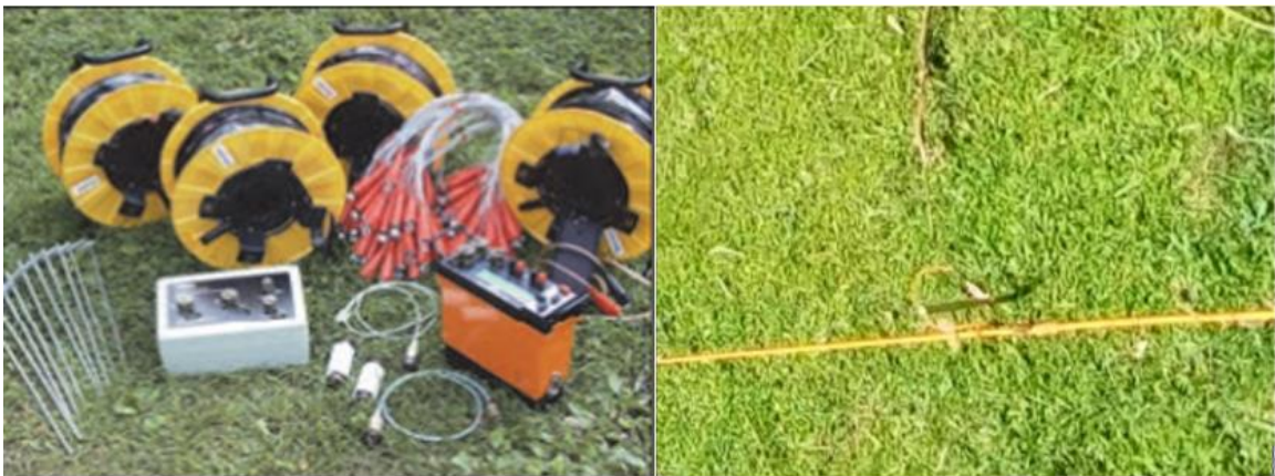
Figure 3.6 Instrument and Electrode Installation of Geo-Electrical Survey
