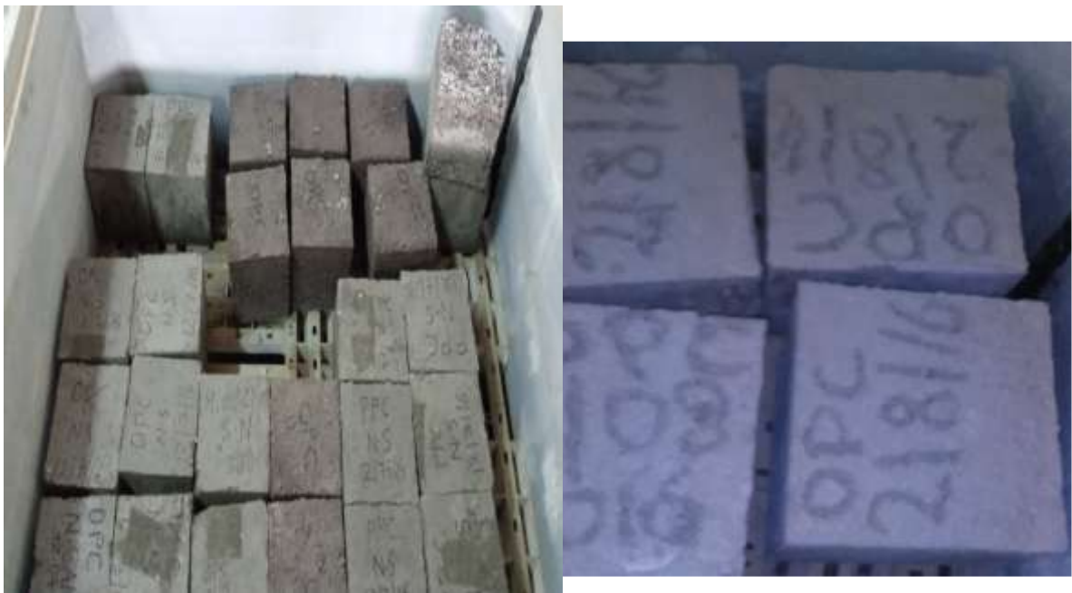
Figure 3.8. Self-curing of concrete
