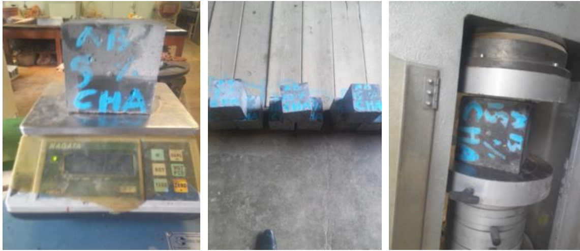
Photo 19 concrete specimen's weight measurement (left), before and during compressive strength test (center and right respectively)
