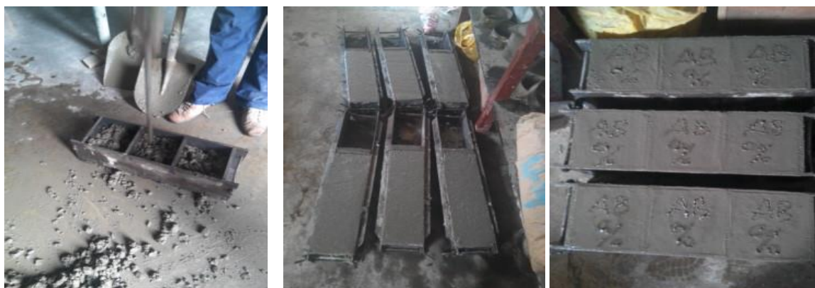
Photo 15 Concrete specimens' preparations being trawled and finished
