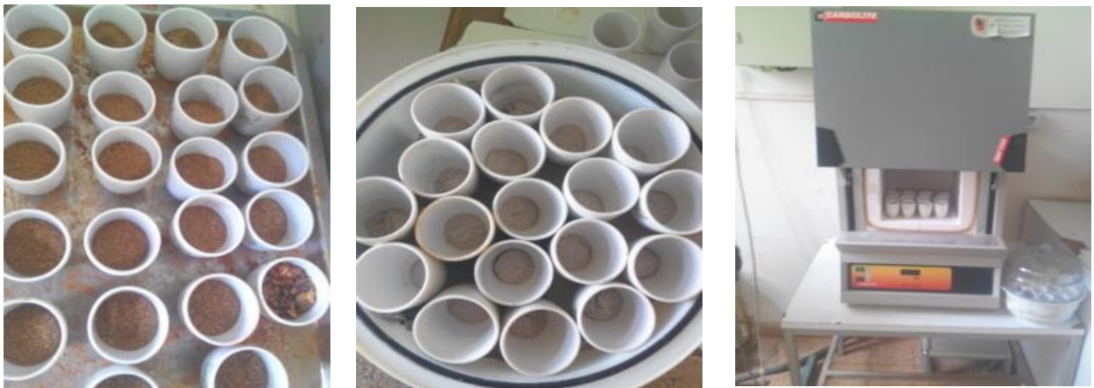
Photo 2 Determination of coffee husk ash by Furness at PH laboratory
