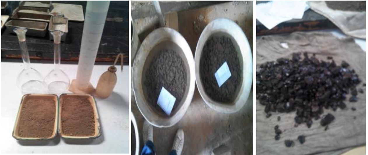
Photo 7 Fine and Coarse aggregate under specific gravity test
