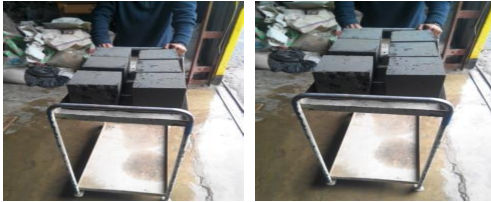
Photo 16 concrete spacemen transported to curing pond after Demolding
