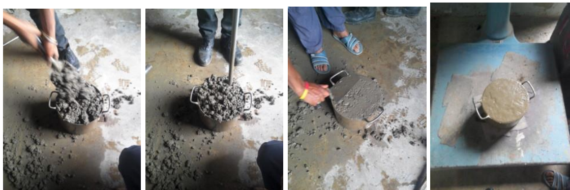
Photo 14 Fresh concrete properties of fresh unit weight test
