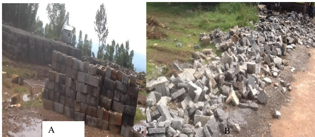
Figure 4-8: Poor handling of HCB during manufacturing and storage at Afro-Tsiyone storage site
