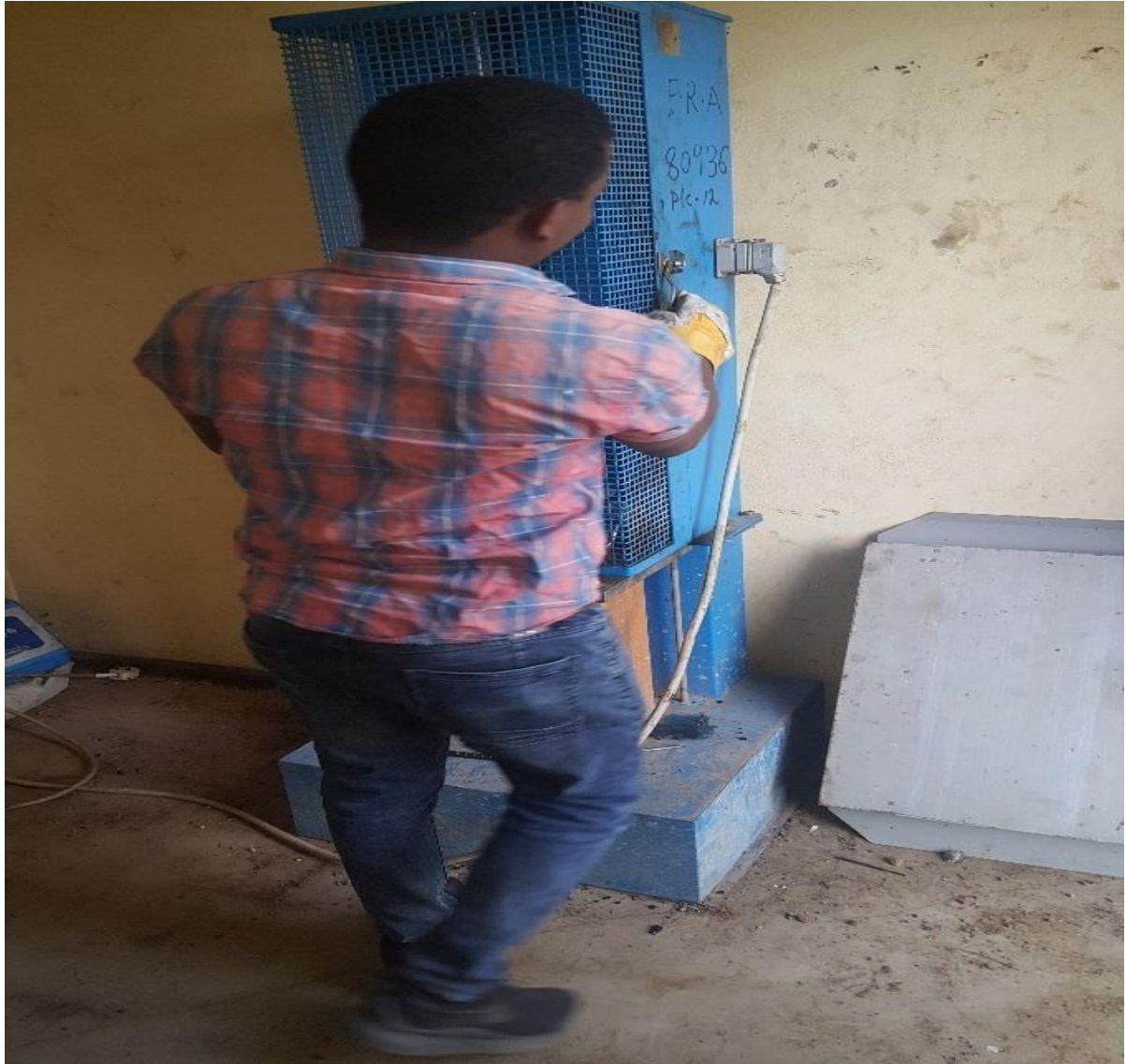
Figure 3.6. Compaction of hot specimen
