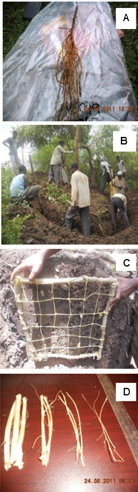
Figure 4. Illustration of the field and lab measurements during root characterization. (A) Horse-tail-type root system of Salix subserrata with numerous thin roots, which help the species to reinforce the soft alluvial flood plain along riverbanks, (B) circular trench excavated to determine root density and root area ratio of Albizia gummifera , (C) profile wall method for determining root area ratio; and (D) root samples of four diameter classes of A. gummifera roots ready for tensile strength measurement. [Colour figure can be viewed at wileyonlinelibrary.com ]
