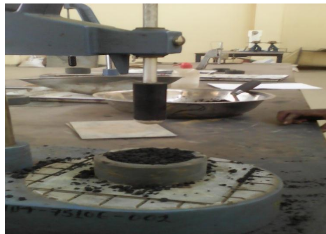
Figure 3.10 Consistency of cement with different percentage of cemen
