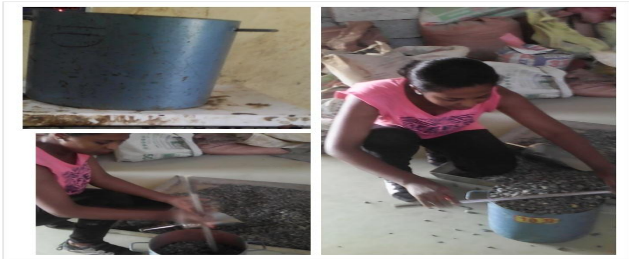
Figure 3.7 The Bulk Density of the Coarse Aggregate Test
