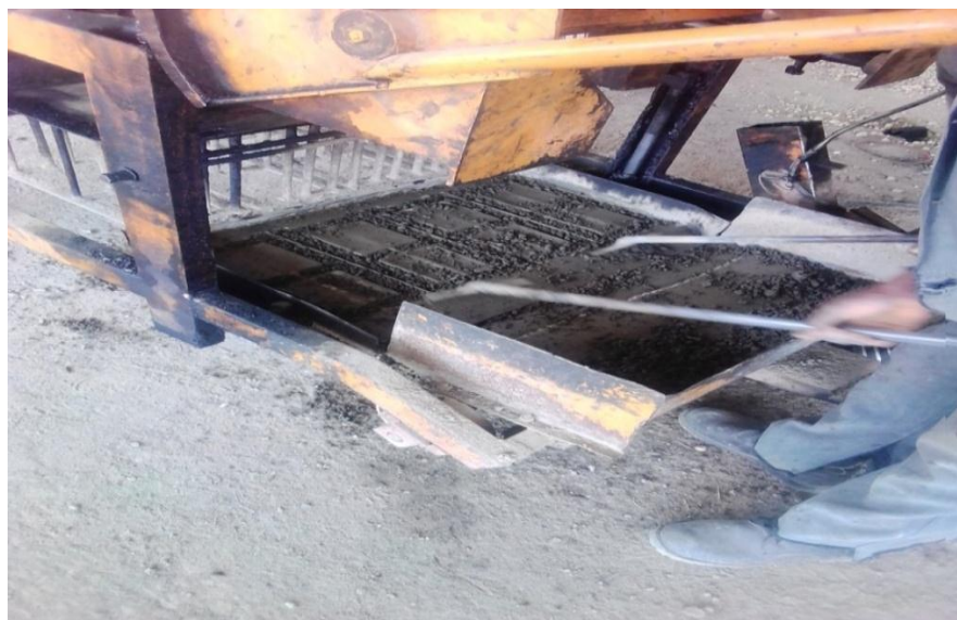
Figure 3.15 Moulding Machine of hollow concrete block
