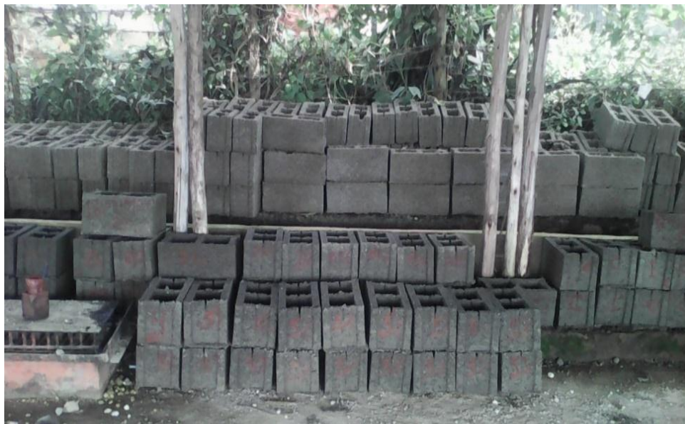
Figure 3.18 Hollow concrete block samples on the production place
