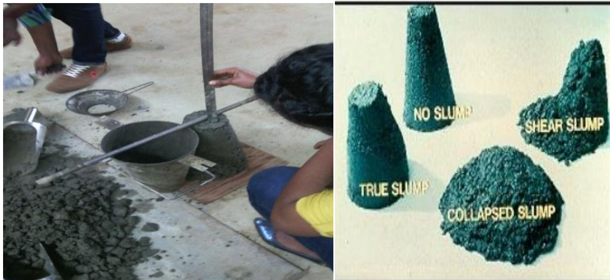
Figure 3.13 measuring slump of fresh concrete mix
