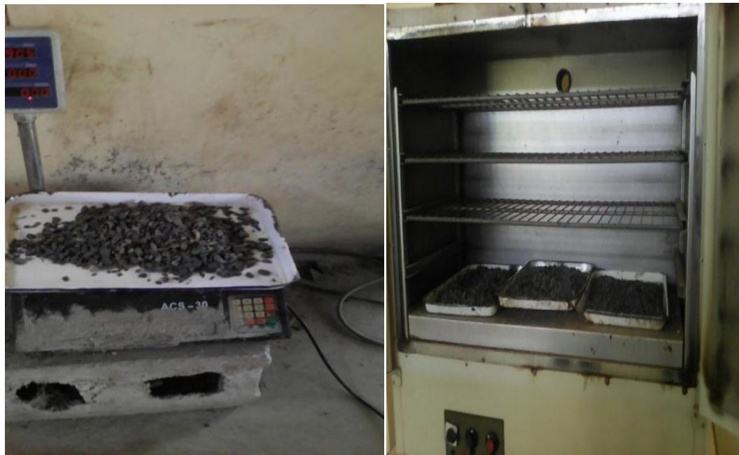
Figure 3.8 Moisture content of coarse aggregate test
