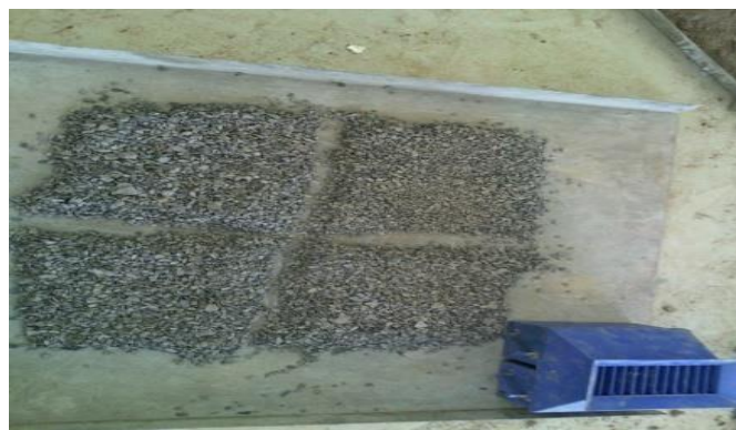
Figure 3.5 Sampling techniques for aggregate
