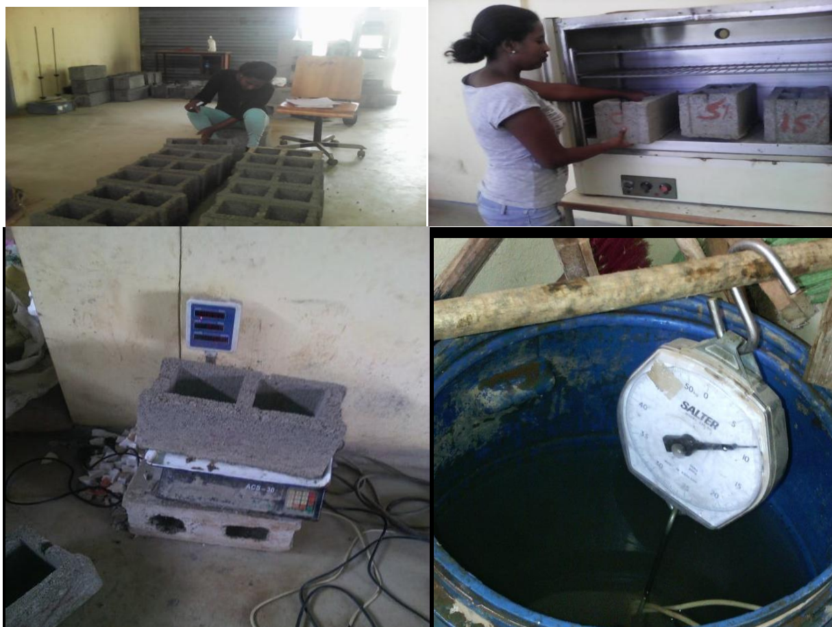
Figure 3.17 Water absorption, Moisture content and Density
