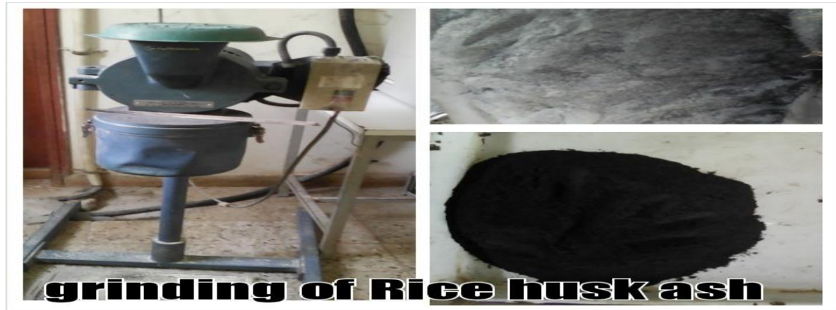
Figure 3.4 Grinding of rice husk ash
