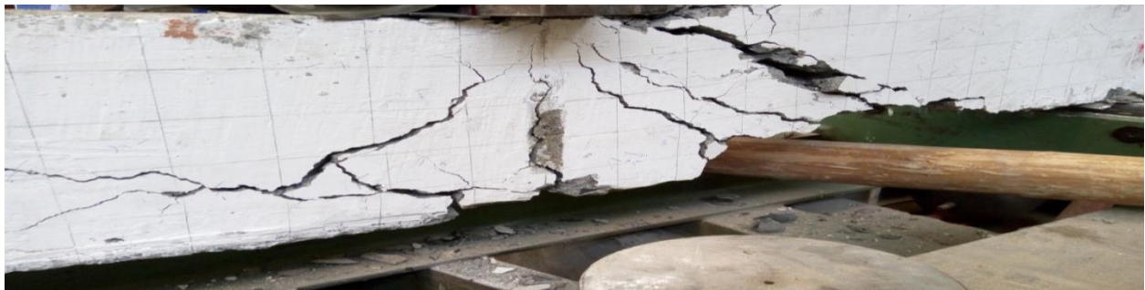
Figure4. 18 Mode of failure for TB-4 under reverse side monotonic loading
