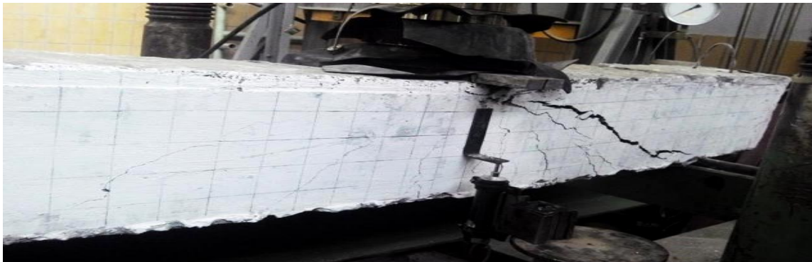
Figure4. 8 Mode of failure for TB-1
