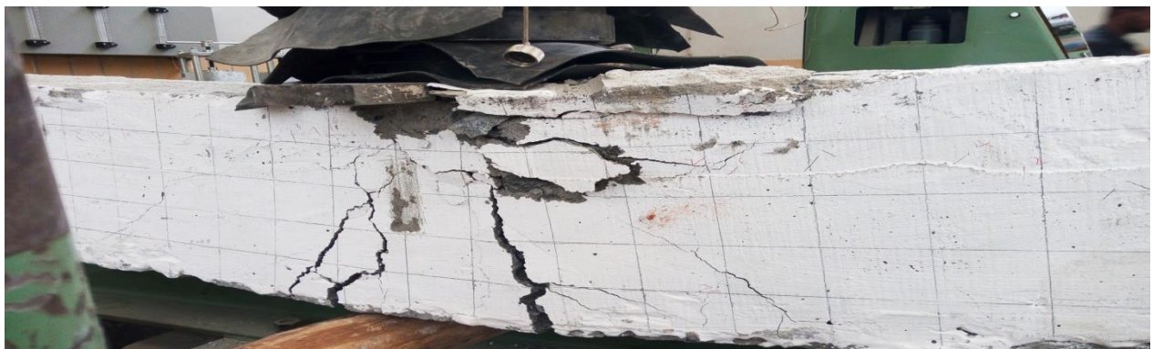
Figure4. 14 Mode of failure for TB-3
