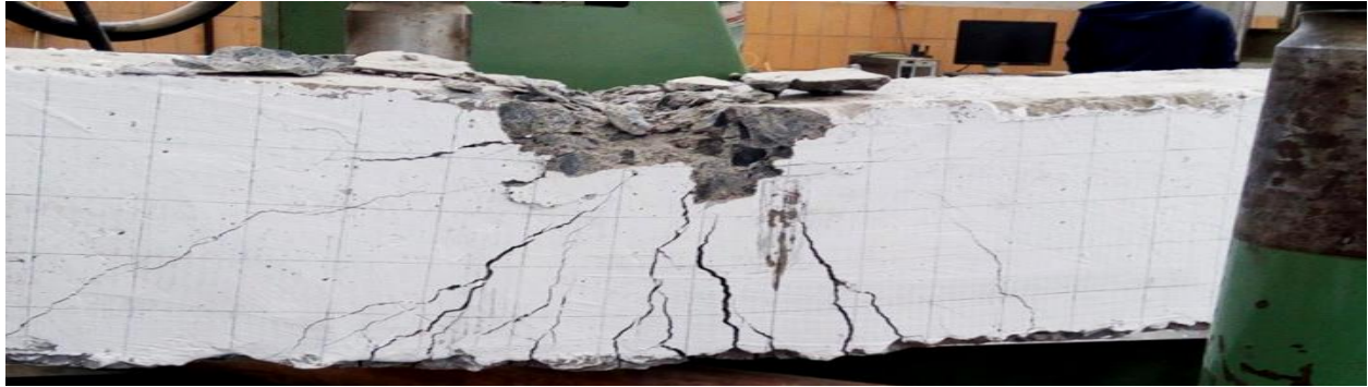
Figure4. 11 Mode of failure for TB-2
