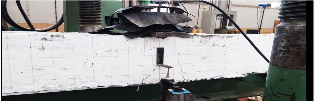
Figure4. 13 Cracks propagation for TB-3
