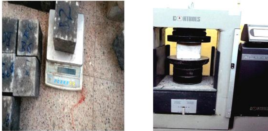
Figure3. 7 Concrete compressive test
