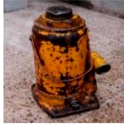
d) Load applying hydraulic jack
