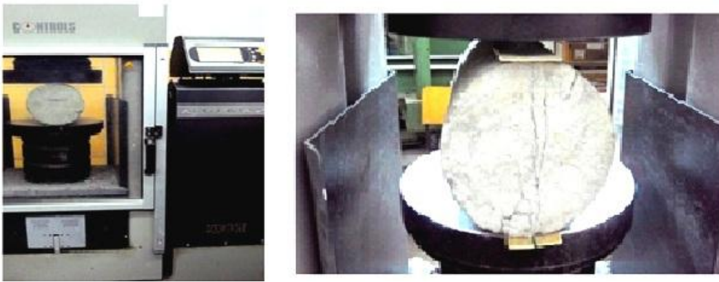
Figure3. 8 Concrete cylinder splitting tensile strength test
