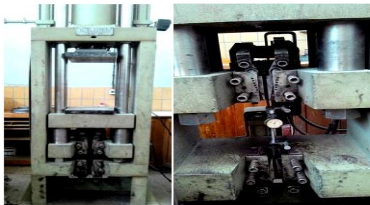
Figure3. 4 Reinforcement Testing Machine
