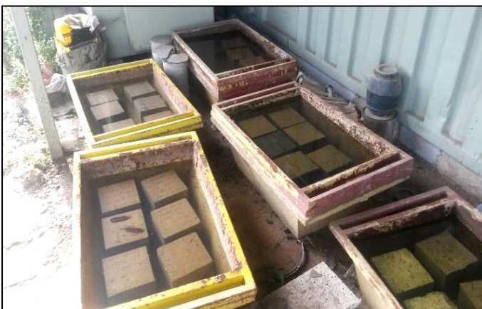
Figure 3.8: Curing of Concrete Cubes
