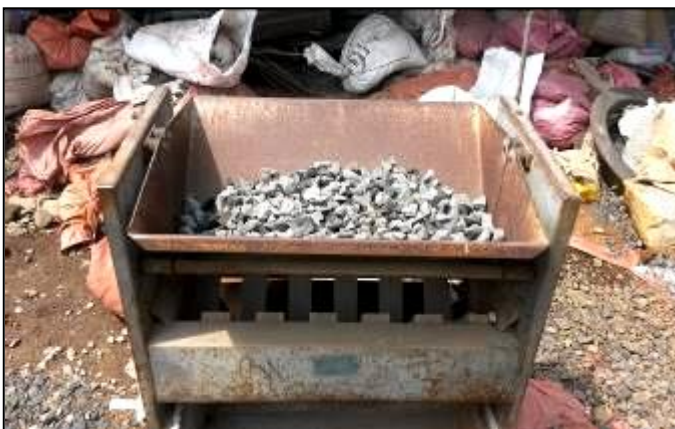
Figure C.1.5: RAC Splitting and Quartering
