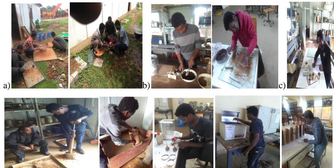
Figure 3.3: a) sieve analysis b) LL and PL test, c) compaction and CBR soaking d) specific gravity test and hydrometer test pictures of laboratory test activities
