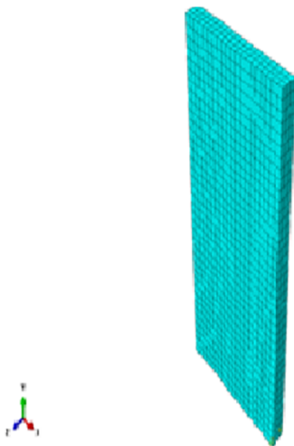
Fig. 3.7a) mesh of cantilver rc shear wall
