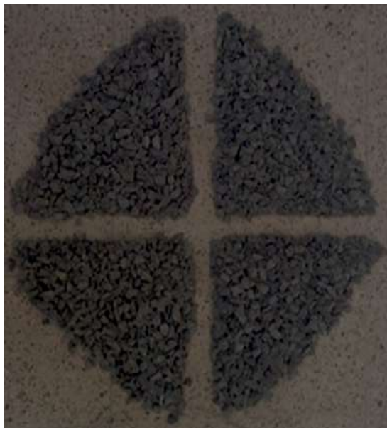
Photo 3: Sample quartering for coarse aggregate (using riffle box on the right).
