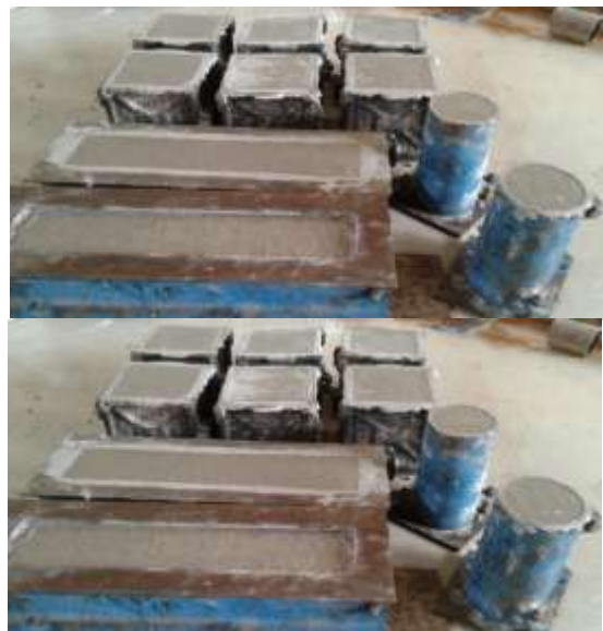
Photo 5: Oiled concrete molds (left) and casted concrete specimens being trowled (right)
