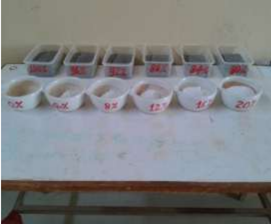
Photo 2: Prepared MDP & OPC at different (%) for blending (right) and slump test (left)
