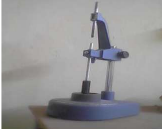
Figure 3.6 Normal consistency testing (Vicat apparatus)
