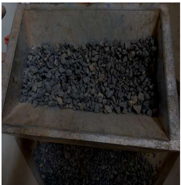
Photo 3: Sample quartering for coarse aggregate (using riffle box on the right).
