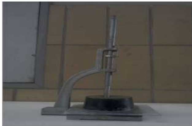
Figure 3.7 Setting time testing (Vicat apparatus)
