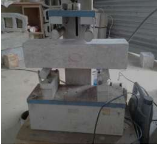
Photo 8: Concrete beams under flexural test on the left and after flexural test on the right
