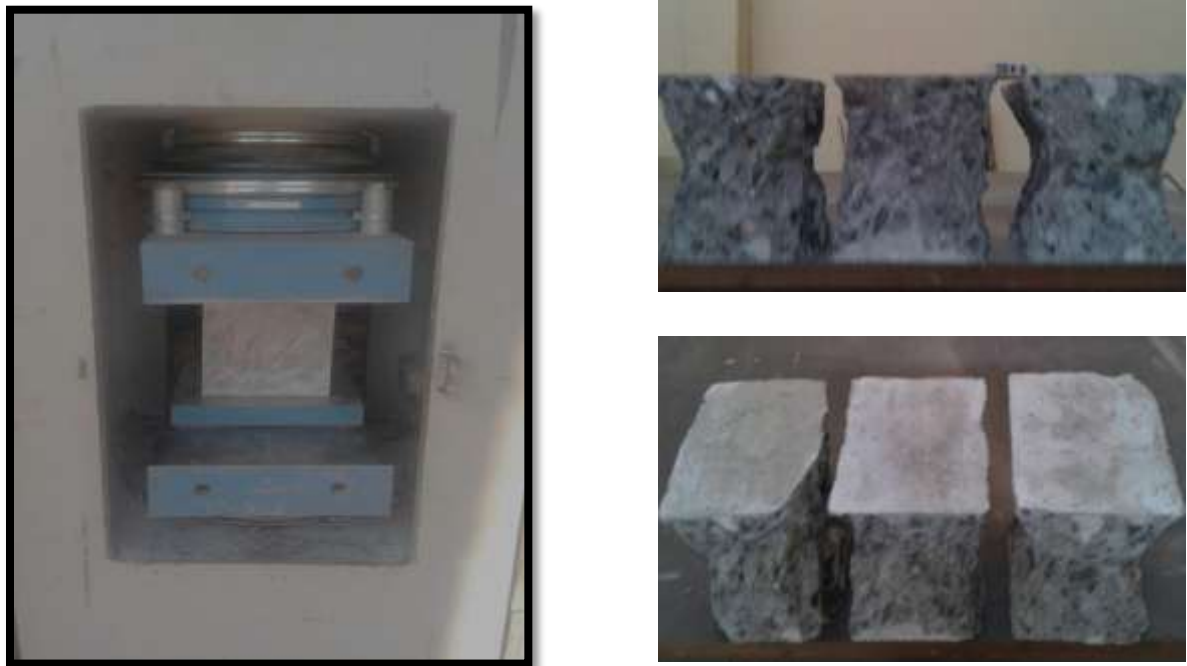
Photo 7: Cubes under compression test on the left and after compression test on the right
