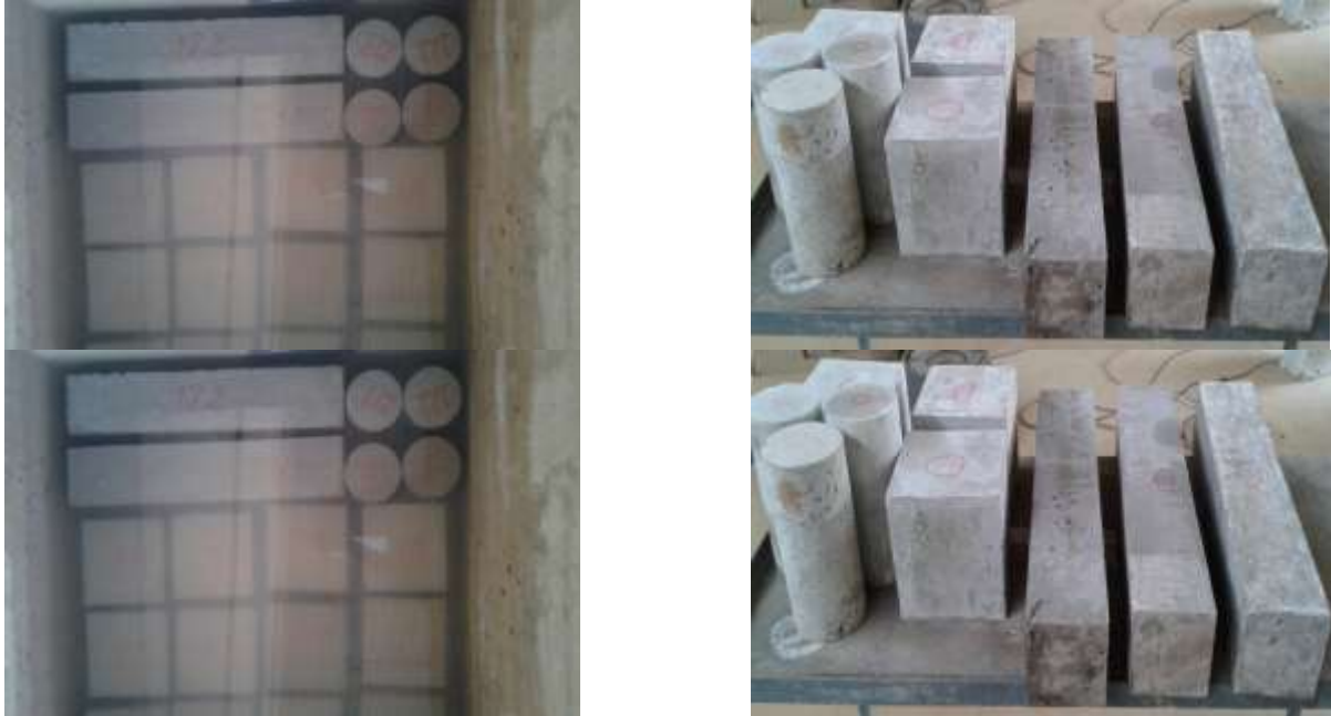
Photo 6: Concrete specimens in curing pond (left) and after curing (right)
