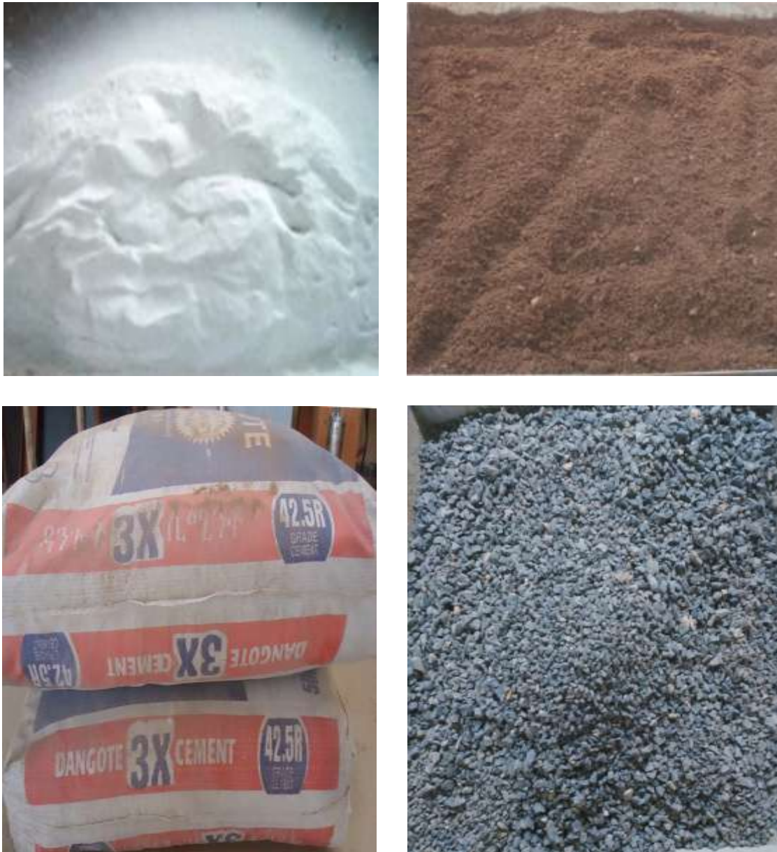
Photo 1: Concrete making materials: marble dust powder (top left), cement (bottom left), sand (top right) and coarse aggregate (bottom right).
