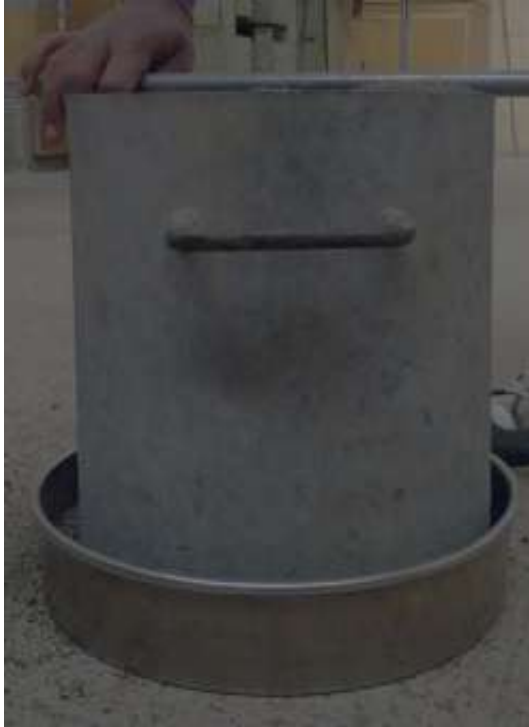
Photo 4: Unit weight test using known volume (left) and sieving MDP using shaker (right)
