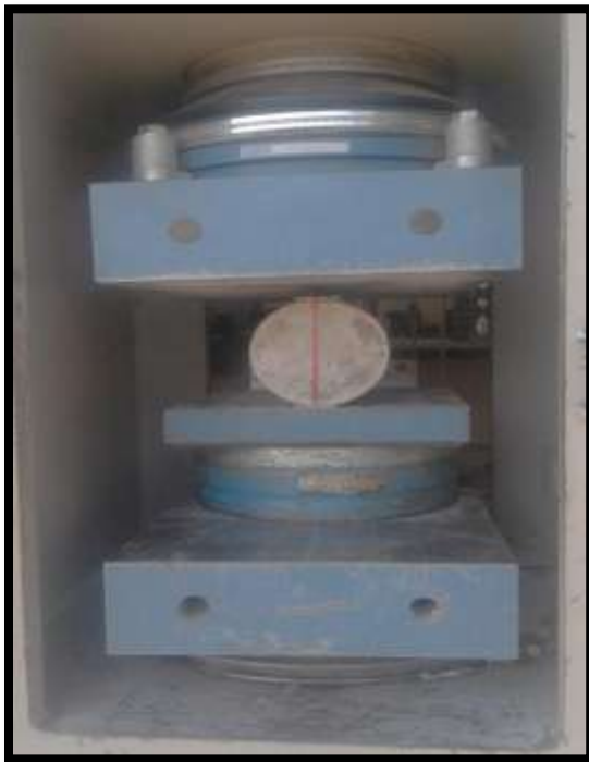
Photo 9: Cylinders under tensile split test on the left and after tensile split test on the right
