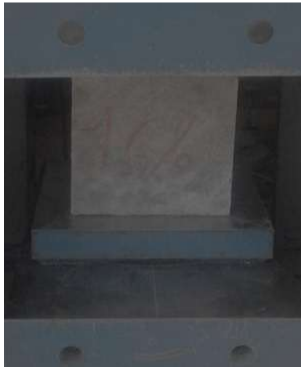
Figure 4.4 Compressive strength of concrete being tested
