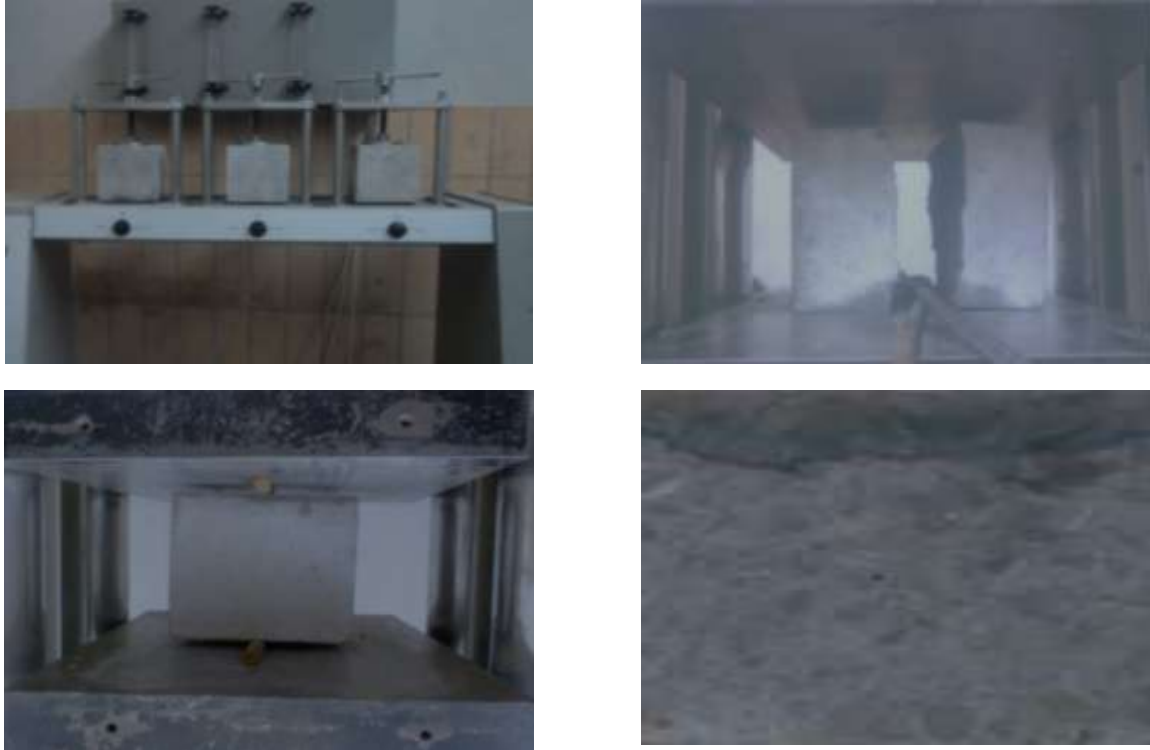
Photo 10: Permeability test: Cubes under the rig (top left), under splitter machine before split (bottom left), after split (top right) and cross sectional view after split (bottom right).
