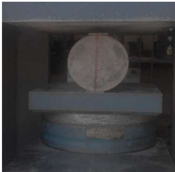
Figure 4.6 Cylindrical specimens under tensile split test
