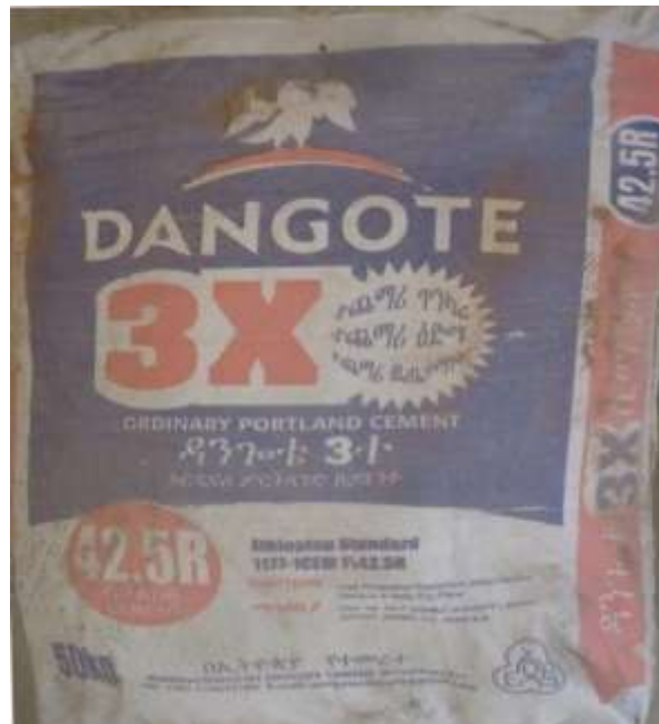
Figure 3.2 Dangote 3x Ordinary Portland cement (OPC) used in the research
