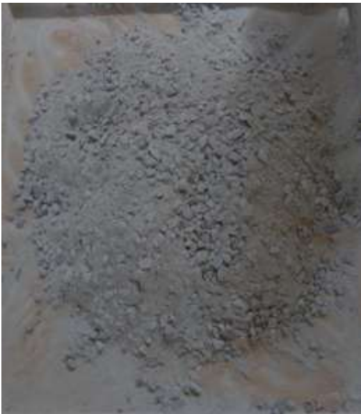
Photo 13: Dry state mix of Coarse and Fine aggregates (on the left) and marble powder added to the dry mix (on the right).
