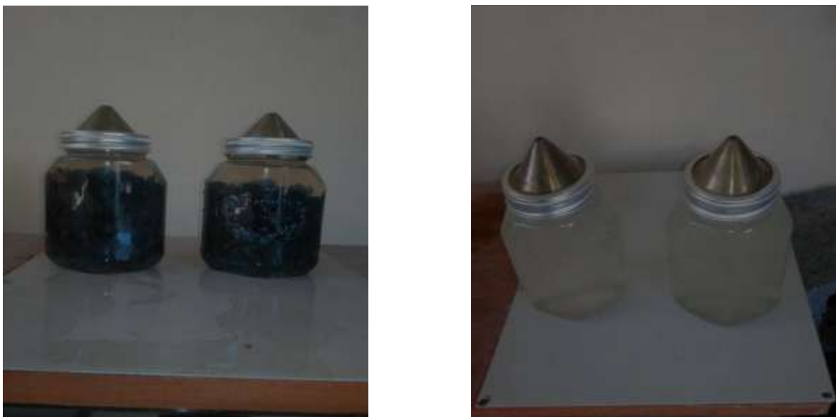
Photo 11: Specific gravity and water absorption test for aggregates by using pycnometer
