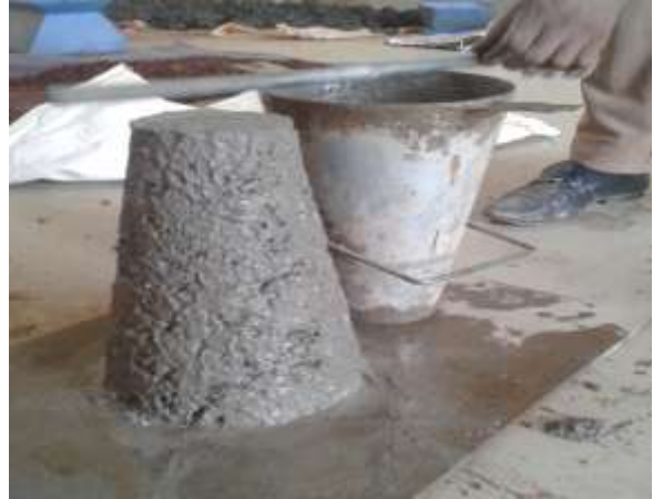
Photo 2: Prepared MDP & OPC at different (%) for blending (right) and slump test (left)
