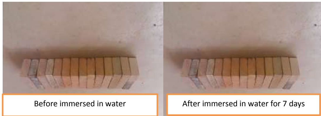
Figure 4.6: Efflorescence test of bricks
