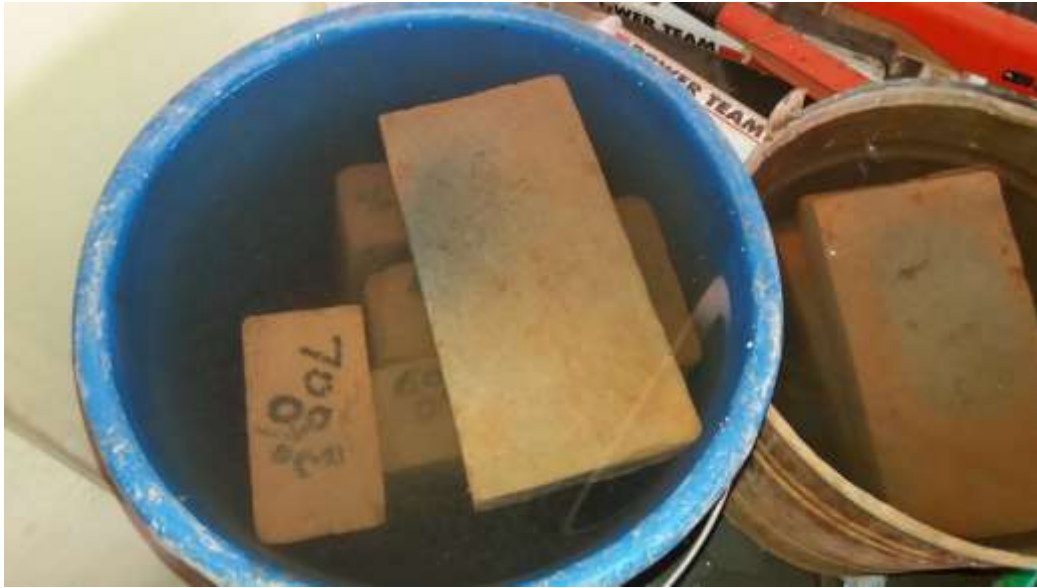
Figure 3.15: Immersing bricks in cold water for 24hrs
