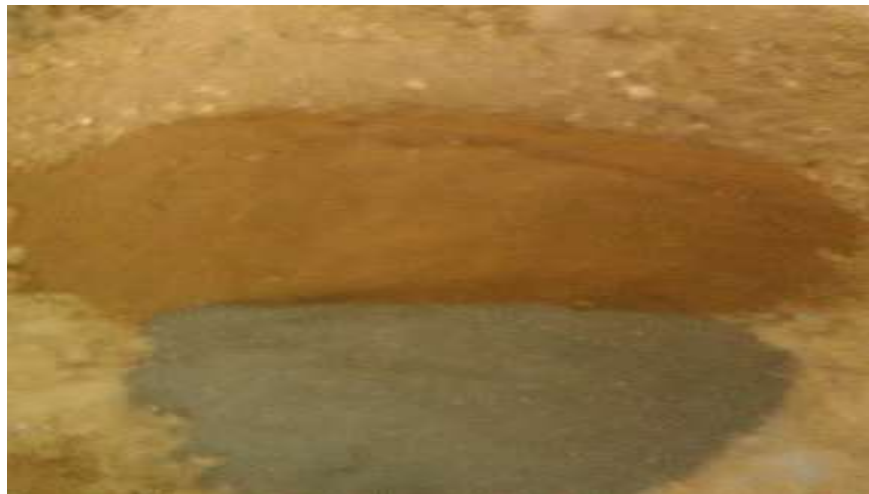
Figure 3.11: Dry mixing the during the production of the bricks sample
