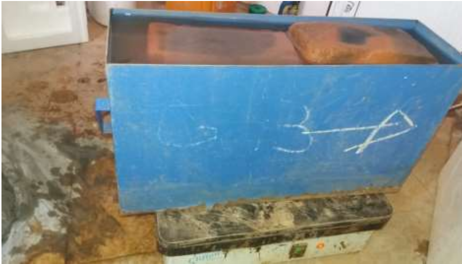
Figure 3.16: Boiling bricks for 5hrs to test water absorption
