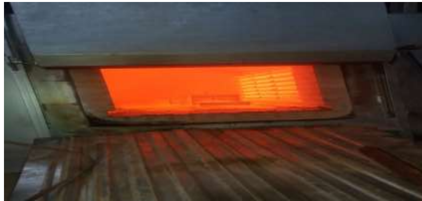
Figure 3.13: picture taken during Firing dried Bricks
