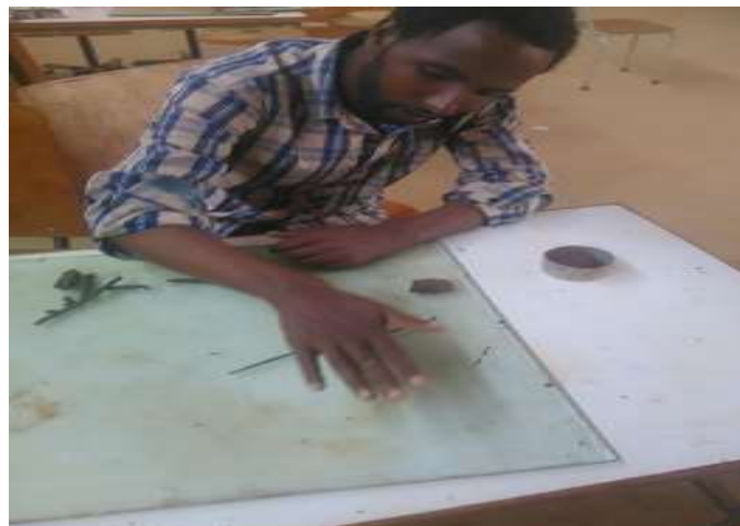
Figure 3.8: Plastic limit test
