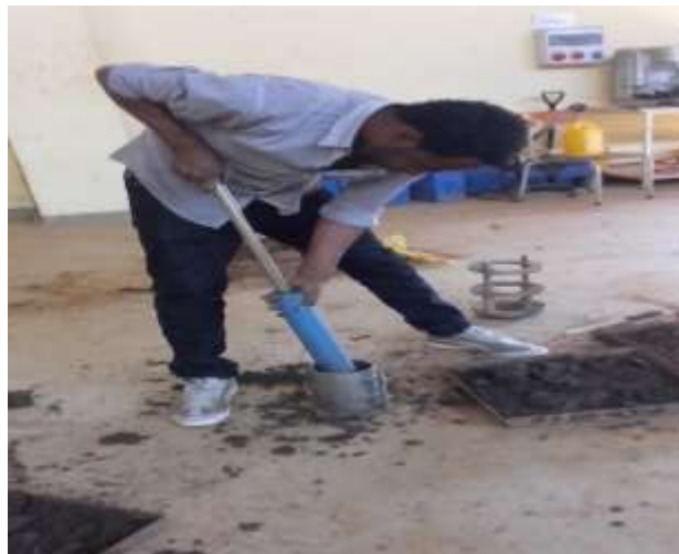
Figure 3.10: photo taken during compaction test
