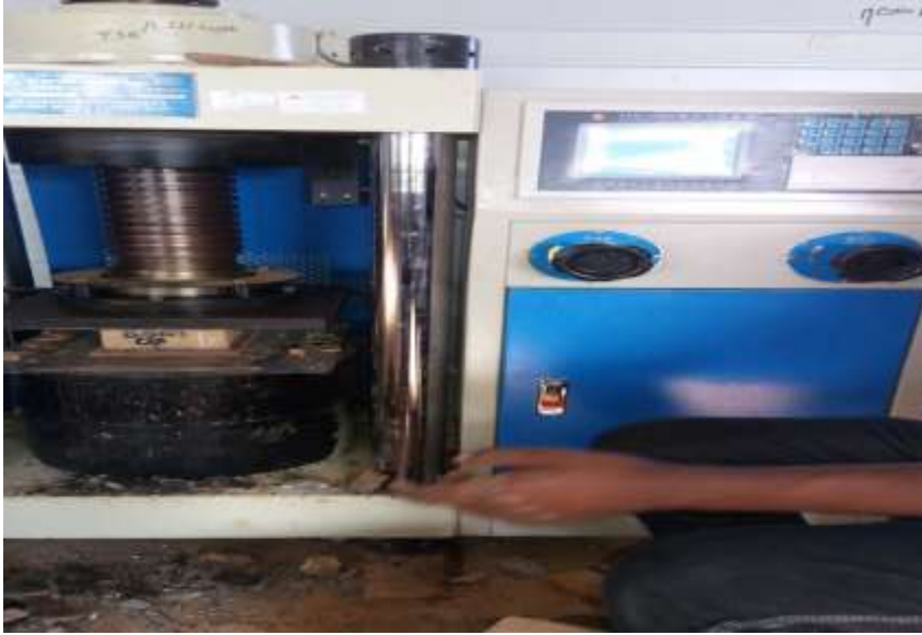
Figure 3.14: Breaking Bricks by using compression machine
