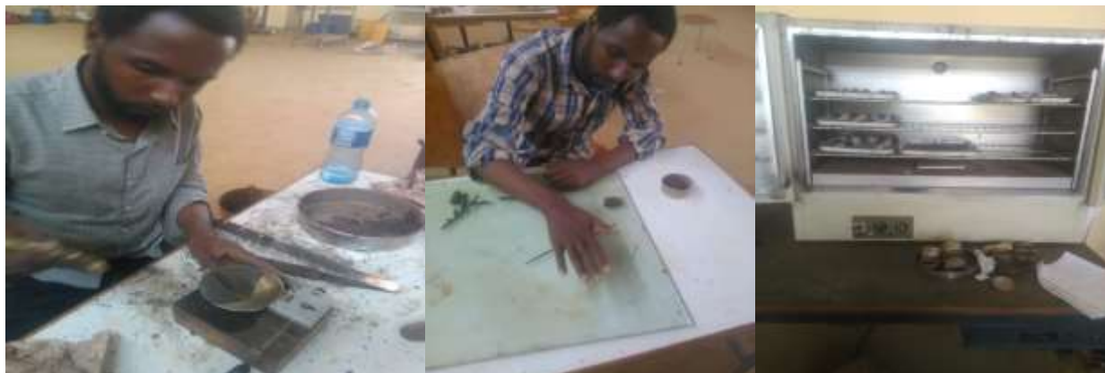
Picture taken during liquid and plastic limit tests
