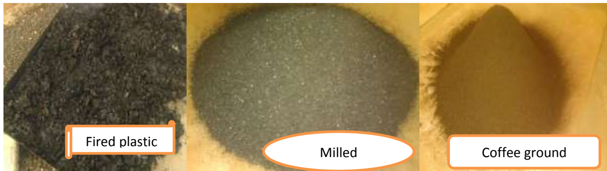
Photo taken during raw material preparation for production of bricks
