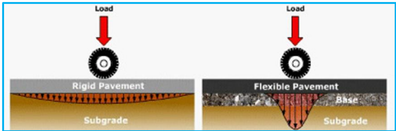
Figure 2.3: Pavement Deflections under a Loaded Wheel (www.loadpavement.com)
