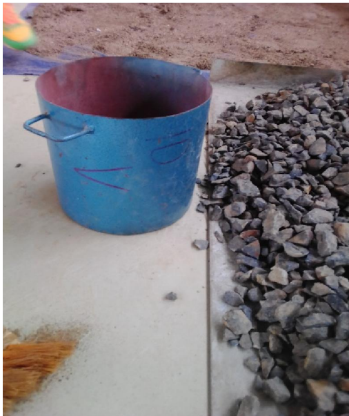
Photo: Unit weight tests
