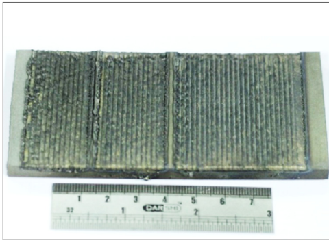
Fig. 9. Pictorial view of laser clad surface before grinding
