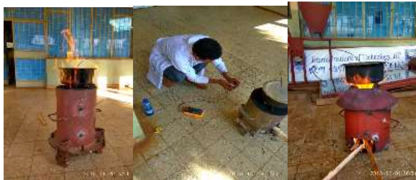
Figure 11: Sample of water boiling test and measuring temperature for the selected stoves
