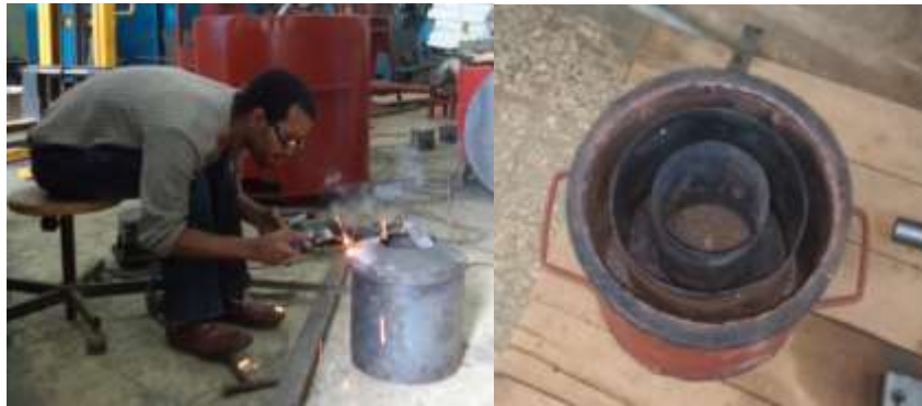
Figure 8: Constructing the continuous feeding biochar producing stove
