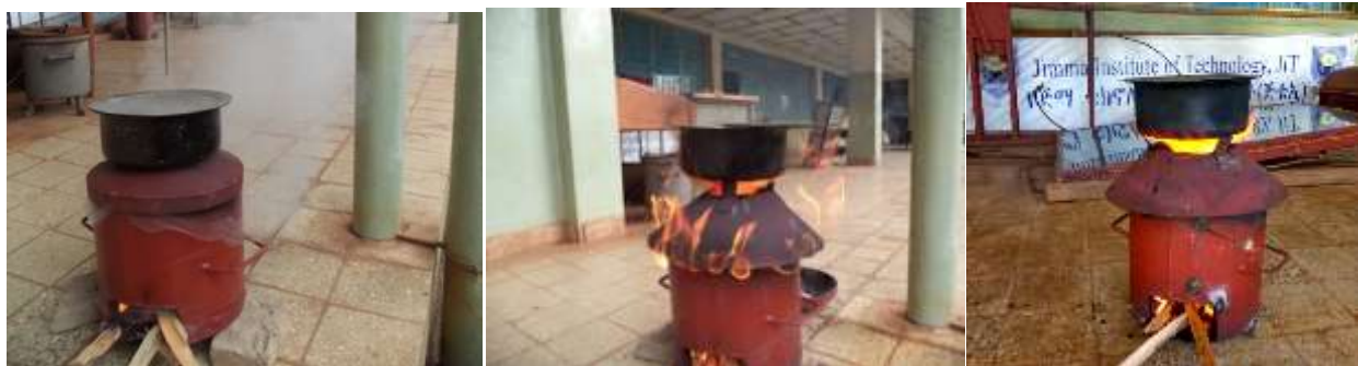
a) without secondary air b) with high inlet of secondary air c) with low inlet of secondary air
