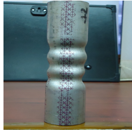
Fig. 5 Roll forming test specimen at a forming pressure of 42 kg/cm 2 .
