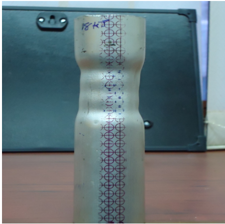
Fig. 3 Electromagnetically deformed tube specimen at a forming energy of 18 kJ.
