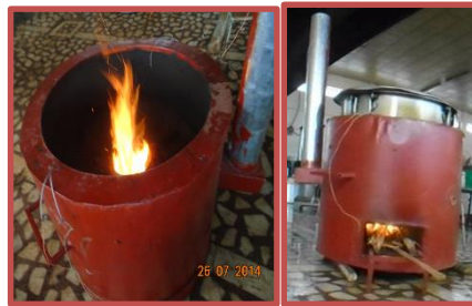
Figure 4.4 InStove during operation
