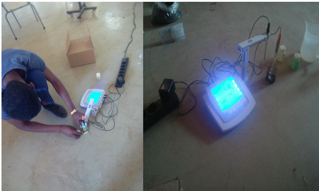
Figure 3.10: Calibration of instrument and measuring biochar sample pH
