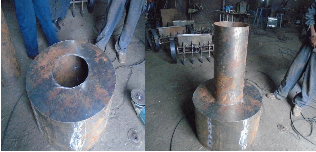
Figure 3.7: a) Up-side down vessel holder b) Assembled vessel holder and combustion cylinder
