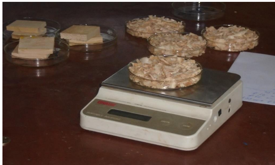
Figure 3.12: Balancing biomass fuel and woodchip sample
