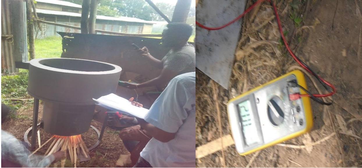
Figure 3.10: Stove temperature test instruments
