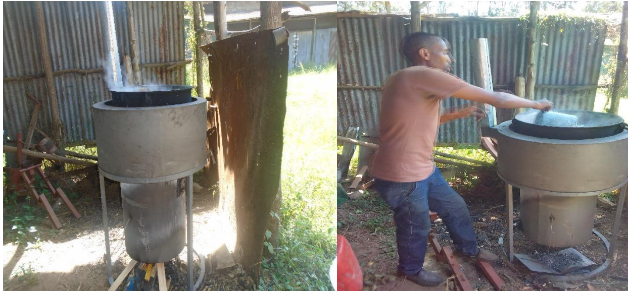
Figure 3.14: WBT of Institutional Bio-char Rocket Stove
