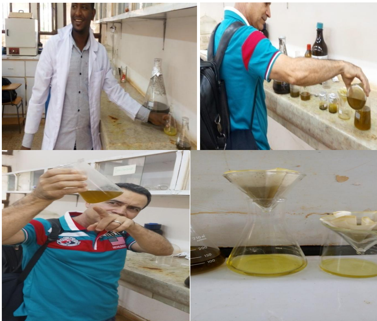
Figure 3.7 Purification of filter mud oil in by using filter paper
