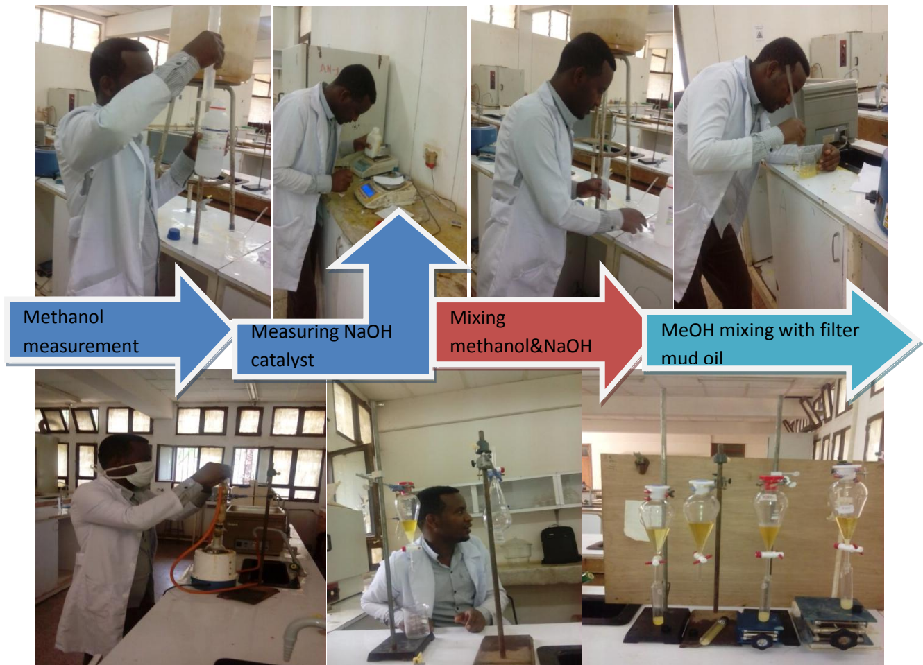
Figure 4.4 Biodiesel production procedure and glycerol separation
