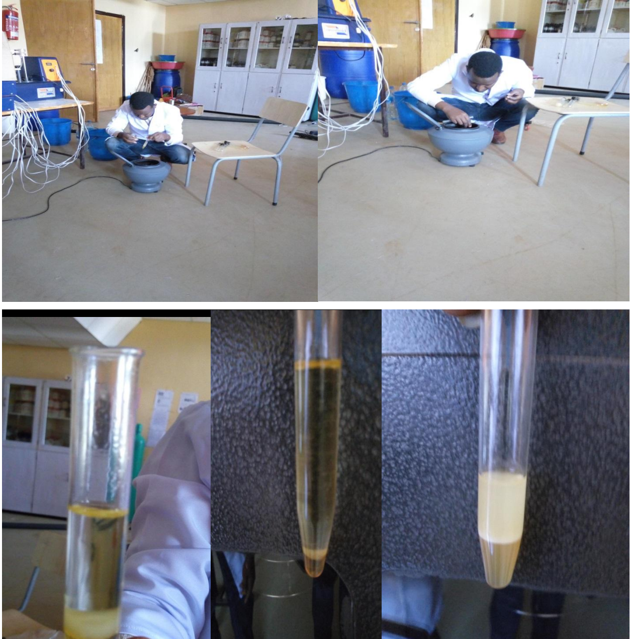
Figure G. Further separation of Biodiesel, residual and glycerin by using centrifugal separation
