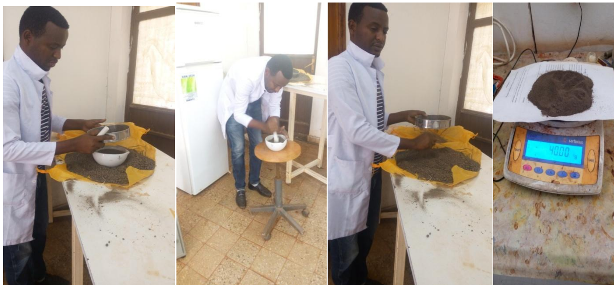
Figure 3.3 Size separations by sieving process and measuring mass for extraction per batch
