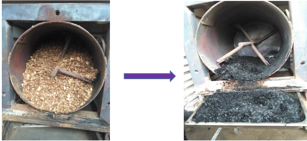
Figure 15. Char from saw dust
