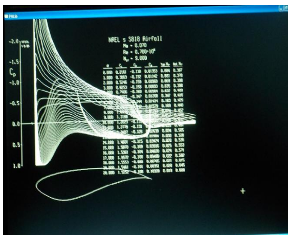
Figure 3 pressure distribution of S818
