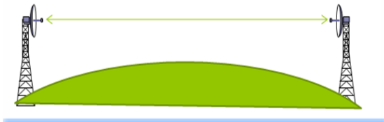
Fig.1. Atypical line of sight microwave link
