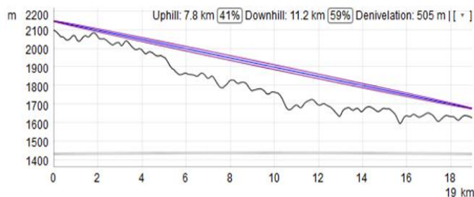
Fig.16. Clearance verification of repeater to site B
