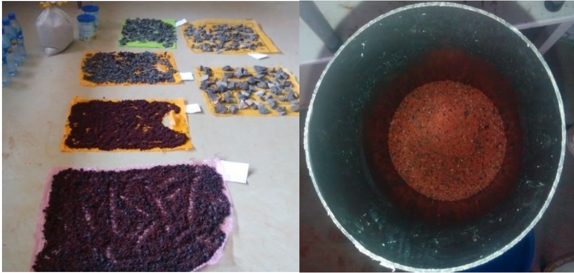
Fig. 4.2. Virgin Scoria after sieve analysis
