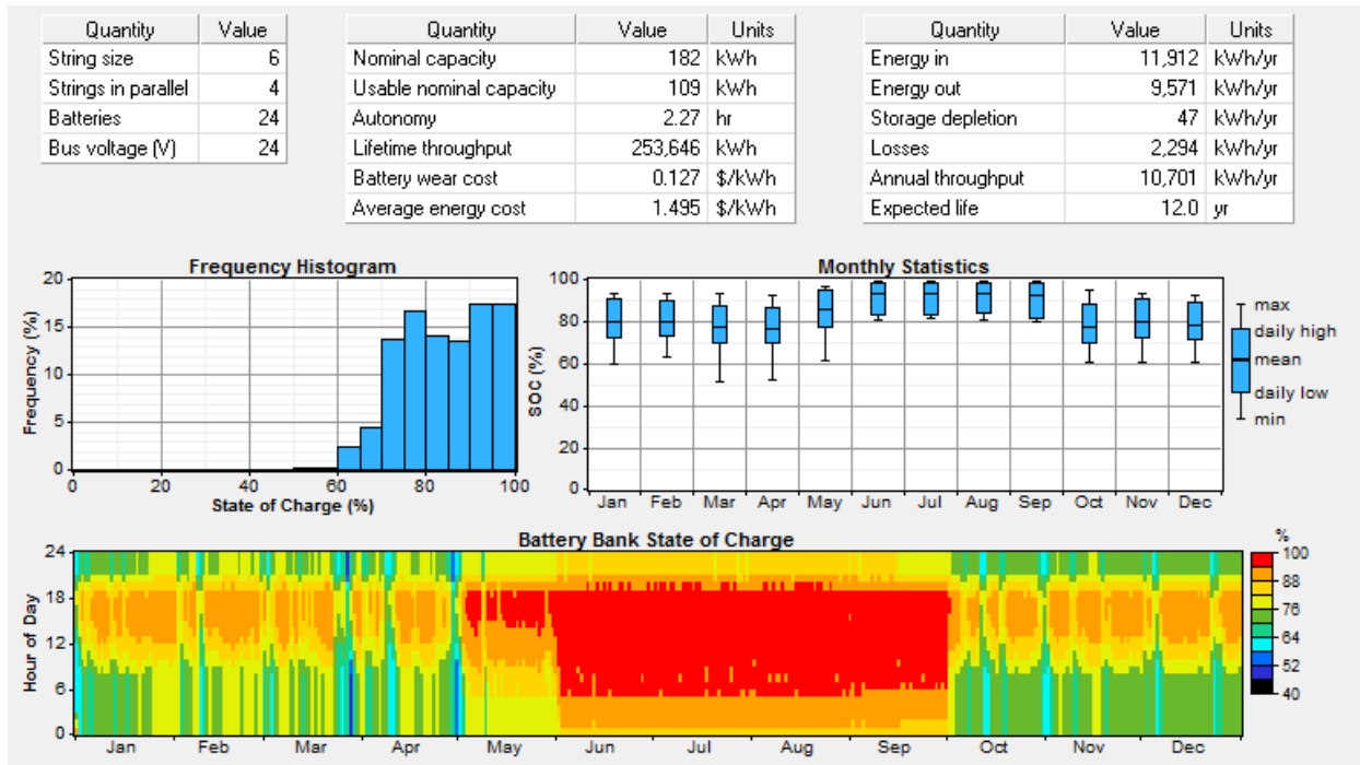
Figure 5.8 State of charge of battery bank
